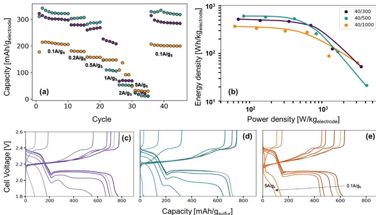
Fig. 6 (a) Rate study of Li-S coin cells from 0.1 A g<sub>sulfur</sub><sup>-1</sup> to 5 A g<sub>sulfur</sub><sup>-1</sup>, (b) the Ragone plot produced from the third cycle of each rate, and (c–e) their corresponding charge–discharge curves.
