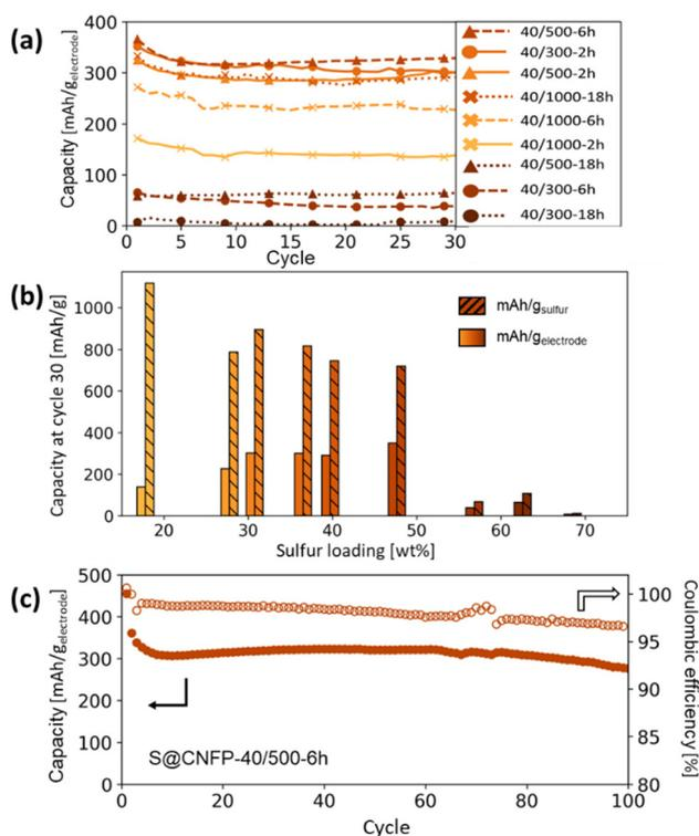
**Fig. 5** (a) Summary of Li-S cycling capacities at 0.1C for CNFPs using different sulfur infiltration durations and (b) their corresponding gravimetric capacities per weight sulfur and per total electrode weight after cycle 30 versus their sulfur weight loadings. (c) Long-term cycling of the S@CNFP-40/500-6 h sample to 100 cycles. Results are summarized in Table S4,<sup>†</sup> and cycling capacity normalized to sulfur mass is shown in Fig. S5.<sup>†</sup>
