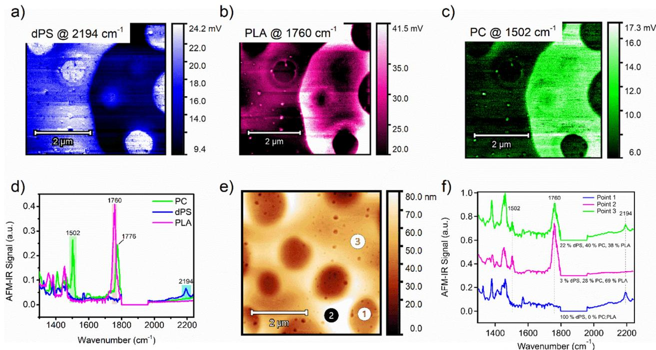
**Fig. 3** (a) Single-band IR imaging of ternary blend of (a) dPS, (b) PLA, and (c) PC. (d) AFM-IR spectrums of PC (green), dPS (blue), and PLA (magenta) with highlighted peaks chosen for single-band AFM-IR scans. (e) Height image of an equal-weighted ternary blend composed of dPS : PLA : PC. (f) AFM-IR spectra of points 1, 2, and 3 indicated in Fig. 3e, with included composition values for dPS, PLA, and PC for those points.
