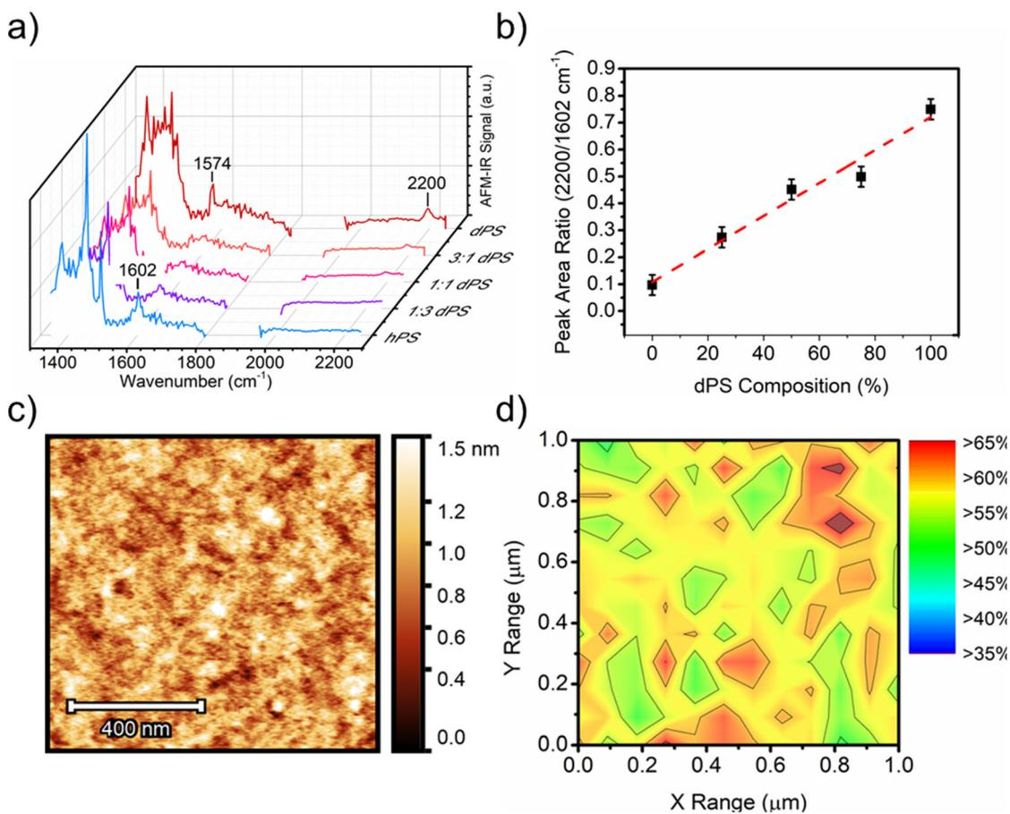
**Fig. 4** Using deuterium to distinguish the isotope polymer blends. (a) Broadband AFM-IR spectrum acquired from dPS:hPS films of different blend ratios. (b) Calibration curve generated from the broadband spectra collected in (a). (c) height image of 1:1 (v/v) dPS:hPS blend. (d) Composition map of area highlighted in Fig. 4c where percentage values indicate dPS fraction.
