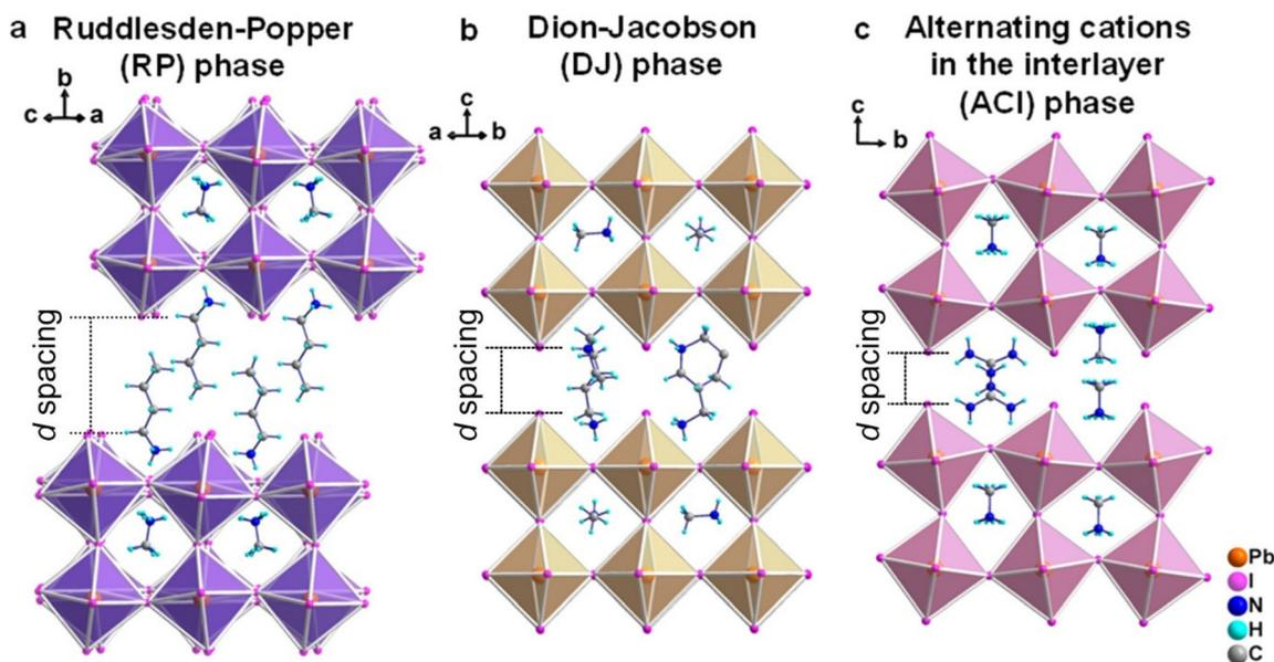
Fig. 2 Lower dimensional layered perovskite structures. (a) The Ruddlesden–Popper (RP) phase, (b) the Dion–Jacobson (DJ) phase, and (c) the alternating cations in the interlayer space (ACI) phase.<sup>21</sup>
