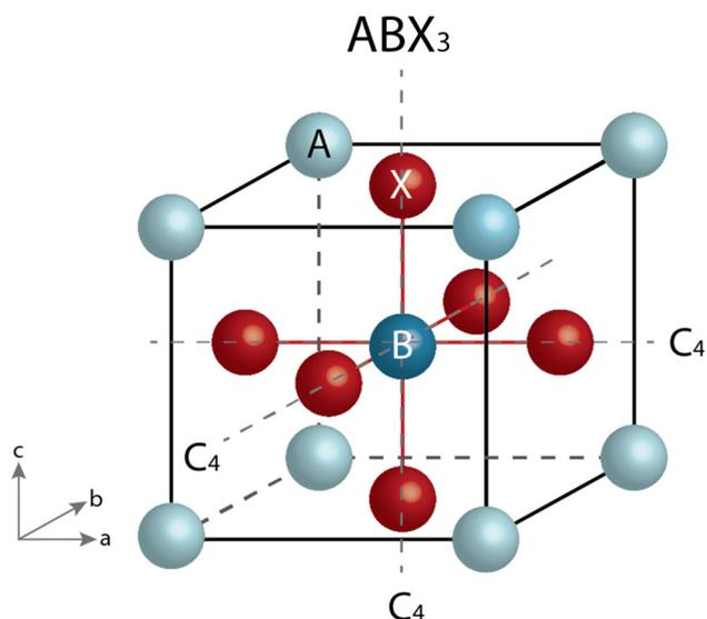
**Fig. 1** The perovskite crystal structure with the molecular formula of  $ABX_3$  (A:  $Cs^+$ ,  $Rb^+$ ,  $MA^+ = (CH_3NH_3)^+$ , or  $FA^+ = (CH(NH_2)_2)^+$ ; B:  $Pb^{2+}$  or  $Sn^{2+}$ ; and X:  $Cl^-$ ,  $Br^-$ , or  $I^-$ ).
