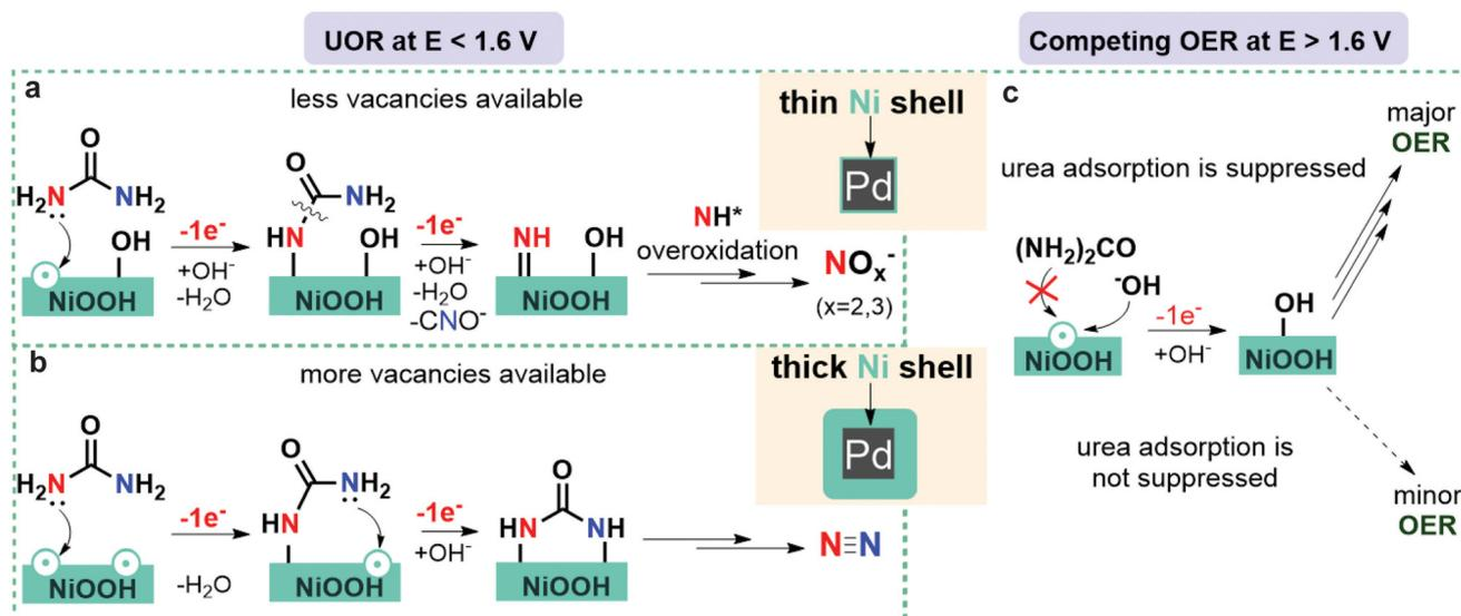
**Fig. 3** The effect of the tensile strain on the UOR mechanistic pathways and competing OER. (a and b) A schematic illustration of the proposed pathways for UOR to  $\text{NO}_x^-$  products (a)  $\text{N}_2$  (b) on the  $\text{NiOOH}$  surface of Pd@Ni NCs with thin shell (a) and thick shell (b) at  $E < 1.6$  V vs. RHE. (c) A schematic illustration of the competition between UOR and OER on the  $\text{NiOOH}$  surface of Pd@Ni NCs with thin shell and thick shell at  $E > 1.6$  V vs. RHE.
