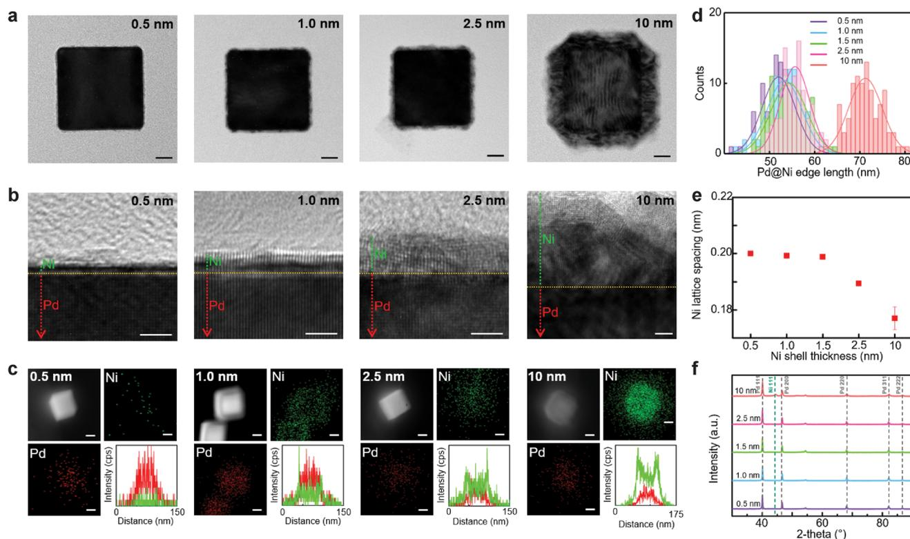
**Fig. 1** Structural analysis of Pd@Ni NCs with different Ni thickness (0.5, 1.0, 2.5, and 10 nm): TEM images (a), HRTEM images (b), elemental mapping (c), edge length distribution (d), Ni lattice spacing (e), and XRD spectra (f). In (b), the dotted green line is a guide for Ni layer, and the dotted red line is a guide for Pd layer. In (c), Ni is indicated in green, and Pd is indicated in red. Scale bars: 10 nm in (a), 2 nm in (b), and 20 nm in (c).
