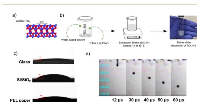
**Fig. 1** (a) Structure of TiO<sub>2</sub>-NS; (b) schematic of the TiO<sub>2</sub>-NS ink formulation process; (c) droplet jetting sequence observed by the Dimatix printer camera; and (d) contact angles of the TiO<sub>2</sub>-NS ink on glass, Si/SiO<sub>2</sub> and PEL-P60 paper substrates, respectively.
