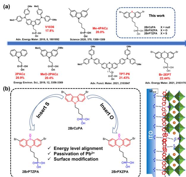
**Fig. 1** (a) Recent development of phosphoric acid-based self-assembled hole-selective materials for inverted perovskite solar cells. (b) Molecular design strategy and chemical structures reported in this work.
