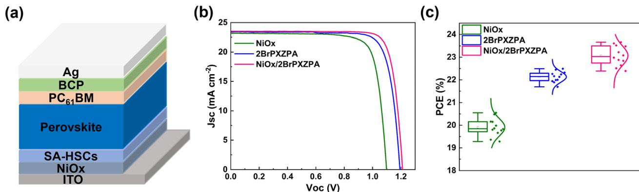
Fig. 5 (a) Schematic diagram of inverted PSC device based on  $\text{NiO}_x$ /SA-HSCs bilayer. (b)  $J$ - $V$  curves of the champion PSC devices and (c) the statistical PCE of PSC devices with different HSCs.
