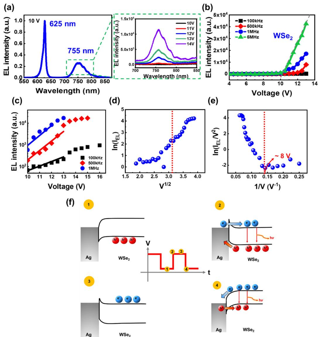
**Fig. 3** (a) EL spectra of the device at various voltages at a fixed frequency ( $\text{WSe}_2$  emission at 1 MHz). (b) Voltage-dependent EL intensity of  $\text{WSe}_2$ . (c) Semi-log plot of the voltage-dependent EL intensity of  $\text{WSe}_2$ . EL intensity–voltage characteristic curves showing (d) Schottky emission and (e) FN emission at the metal– $\text{WSe}_2$  interface. (f) Schematic band diagram of the metal– $\text{WSe}_2$  interface upon a change in polarity of the AC voltage.
