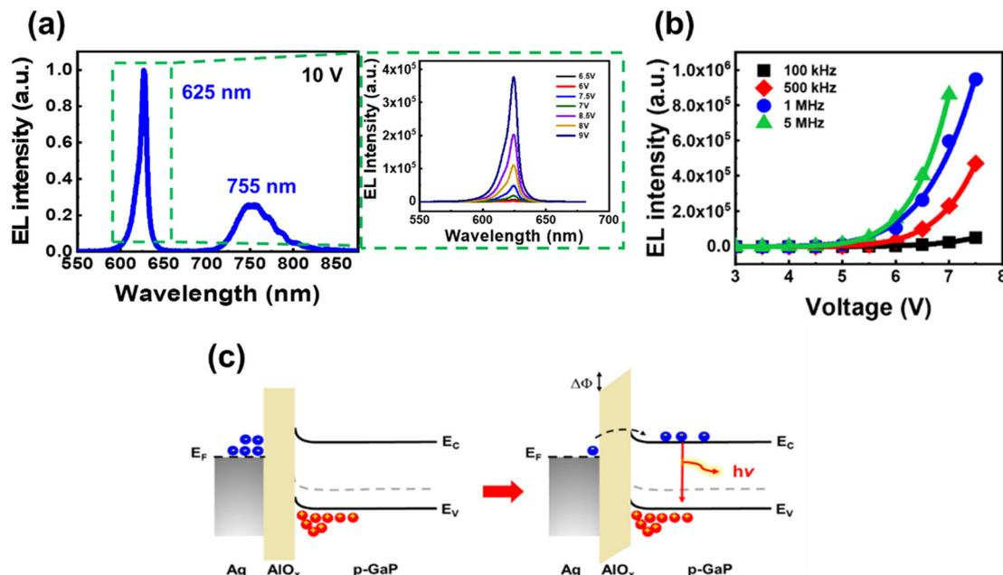
**Fig. 4** (a) EL spectra of the device at various voltages at a fixed frequency (AlGaInP-based MQW emission at 1 MHz). (b) Voltage-dependent EL intensity of AlGaInP-based MQWs. (c) Energy band diagram of the MIS structure of Ag–AlO<sub>x</sub>–p-GaP under zero bias and high bias conditions.
