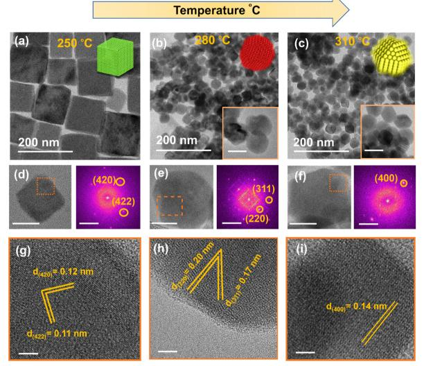
Fig. 2 (a-c) TEM images of NaSbS<sub>2</sub> NCs formed at 250, 280 and 310 °C, respectively the scale bar in the inset images is 50 nm. (d-f) are the magnified images (scale bar is 50 nm) and FFT patterns. (g-i) magnified images of NaSbS2 NCs. The scale in panels (g-i) is 5 nm respectively.
