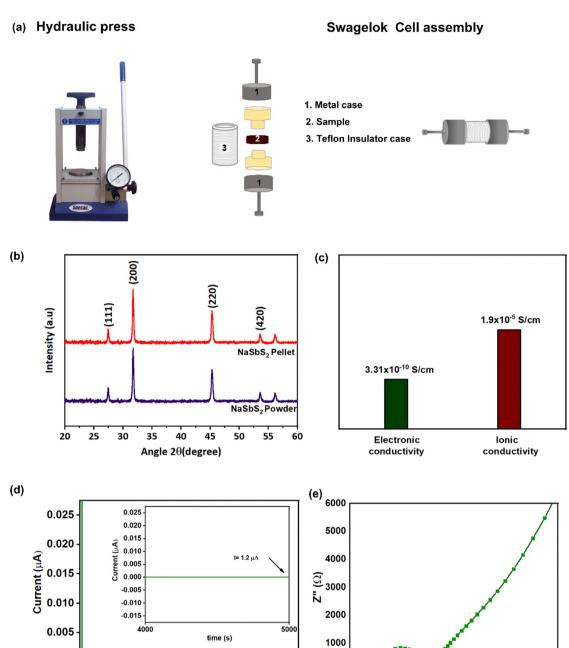
Fig. 6 (a) Schematic for Swagelok cell assembling (b) XRD pattern of the pellet and powder  $NaSbS_2$  before and after cold press (c) bar graph of electronic and ionic conductivity (d) DC polarization of  $NaSbS_2$  with inset showing the current behaviour for duration of 5000 s (e) Nyquist plot of Electrochemical Impedance Spectroscopy (EIS) of  $NaSbS_2$  pellet.
