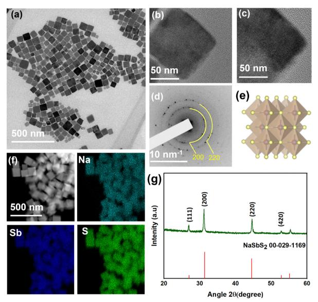
Fig. 1 TEM image (a) of NaSbS<sub>2</sub> NCs with (b and c) tilted TEM imaged at an angle of  $\pm 30^{\circ}$  with (d) SAED and (e) crystal structure showing mixed cation sites of NaSbS<sub>2</sub> yellow (S), red (Na) and blue (Sb). (f) EDX elemental mapping for distribution of the three elements and (g) XRD pattern showing match to cubic phase NaSbS<sub>2</sub> (00-029-1169).
