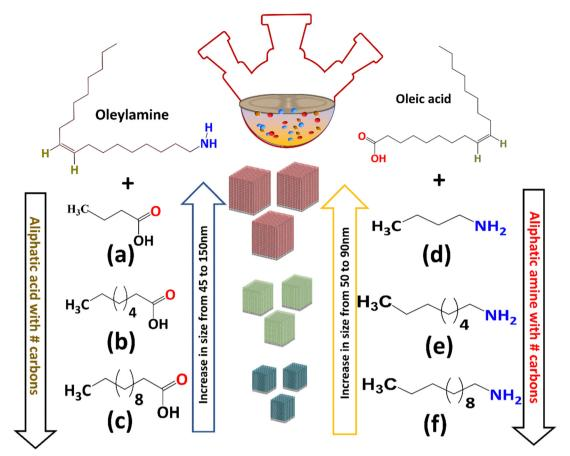
Schematic illustration of the size dependence on the chain length of carboxylic acids (a-c) and amines (d-f)
