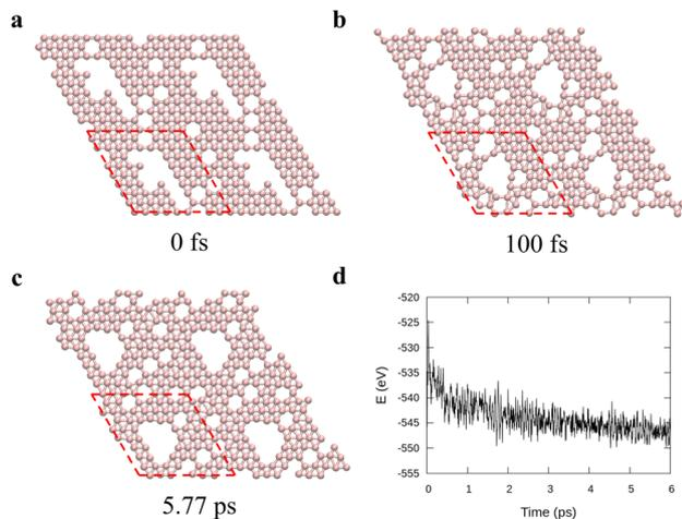
Fig. 6 *Ab initio* molecular dynamics for a  $10 \times 10$  borophene supercell during cooling from 2400 K to 1800 K with  $0.1 \text{ K fs}^{-1}$  cooling rate. (a)–(c) Borophene configurations at specific times: (a) initial, (b) 100 fs, and (c) 5.77 ps and (d) the potential energy during the cooling. Here the red dashed lines denote the unit cell used in the simulations.
