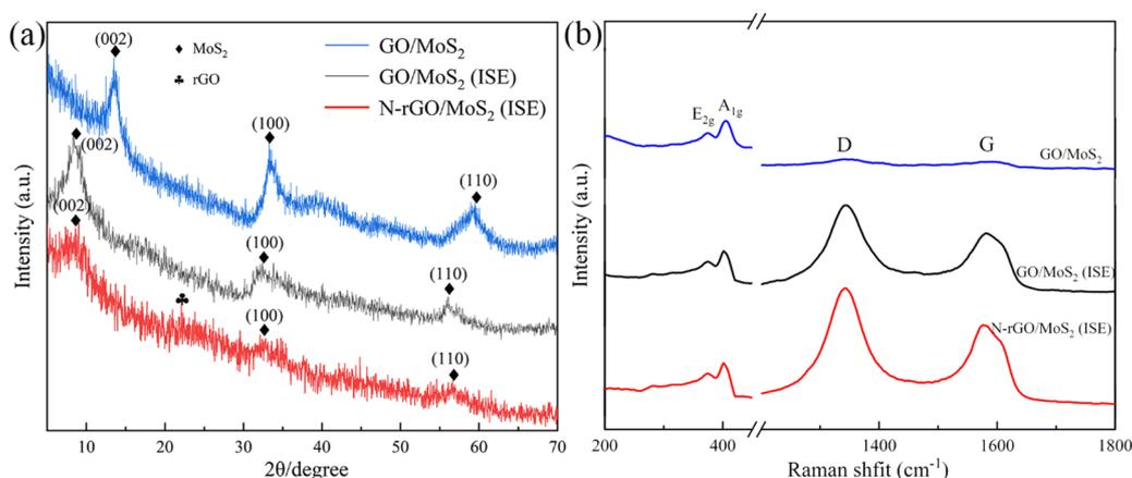
Fig. 1 (a) XRD patterns and (b) Raman spectra of GO/MoS<sub>2</sub>, GO/MoS<sub>2</sub>(ISE) and N-rGO/MoS<sub>2</sub>(ISE).
