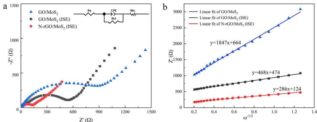
Fig. 6 (a) EIS spectra of GO/MoS<sub>2</sub> (ISE) and N-rGO/MoS<sub>2</sub> (ISE) (inset is equivalent circuit); (b) the linear fits of  $Z'$  and  $\omega^{-1/2}$  of GO/MoS<sub>2</sub> (ISE) and N-rGO/MoS<sub>2</sub> (ISE).
