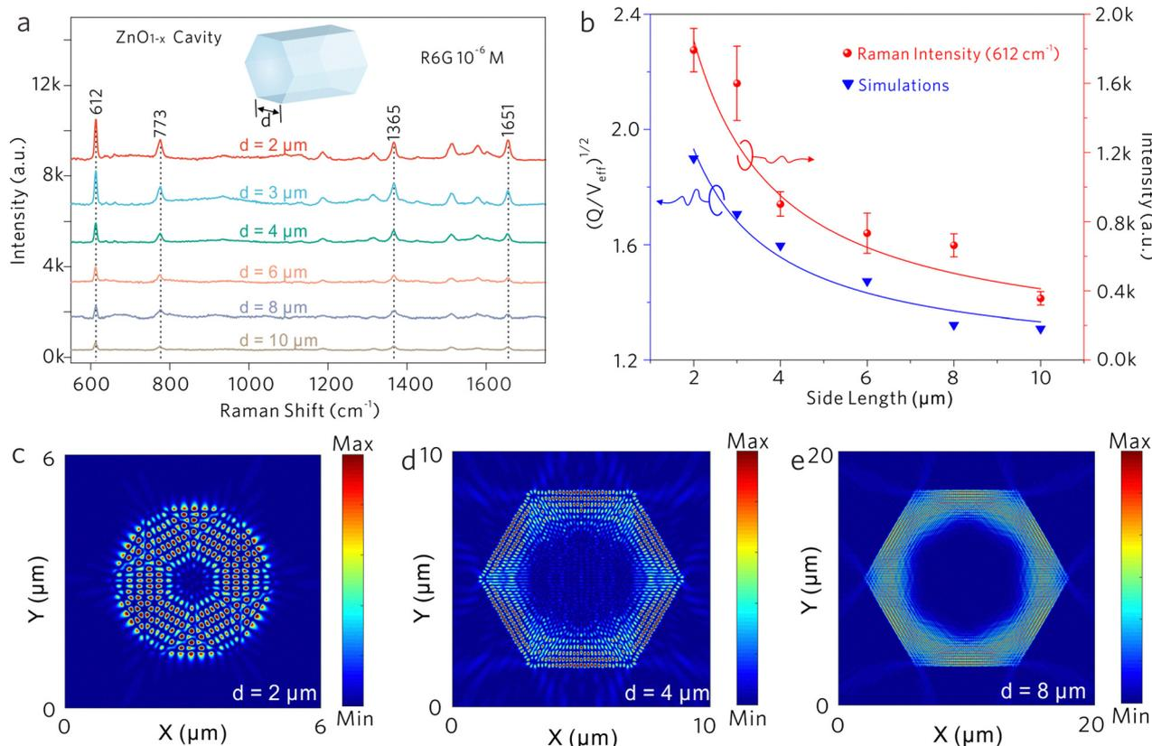
Fig. 5 WGM cavity sensing mechanisms: Purcell effect. (a) Raman spectra of R6G molecules acquired on ZnO<sub>1-x</sub> cavities with different  $d$  values. (b) The relationships of Raman intensities versus side length, and the  $(Q/V_{\text{eff}})^{1/2}$  values versus the side length. Electrical field distribution of the fundamental mode in the X-Y plane from different ZnO<sub>1-x</sub> cavities: (c)  $d = 2 \mu\text{m}$ , (d)  $d = 4 \mu\text{m}$ , and (e)  $d = 8 \mu\text{m}$ .
