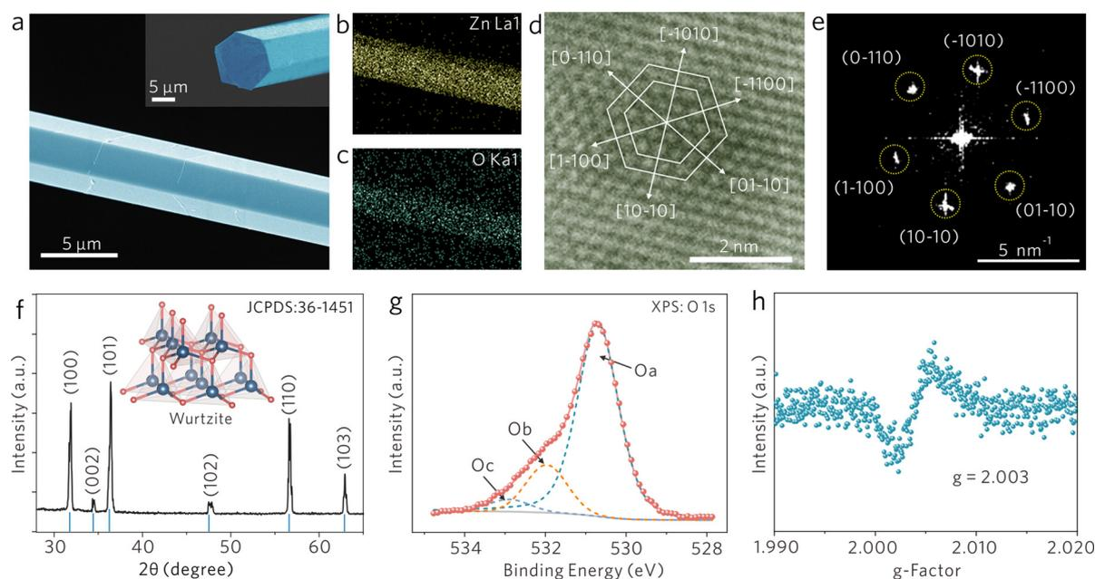
**Fig. 1** Characterization of the  $\text{ZnO}_{1-x}$  WGM cavity. (a) SEM image of the  $\text{ZnO}_{1-x}$  cavity. Inset: the hexagonal cross-section of the  $\text{ZnO}_{1-x}$  cavity. (b and c) Elemental mapping images of Zn and O of the  $\text{ZnO}_{1-x}$  cavity shown in (a). (d) HR-TEM image and the corresponding (e) SAED patterns of  $\text{ZnO}_{1-x}$ . (f) XRD and (g) XPS spectrum of the  $\text{ZnO}_{1-x}$  cavity. (h) EPR spectrum of the  $\text{ZnO}_{1-x}$  cavity.
