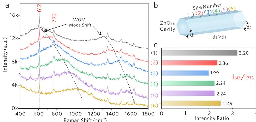
Fig. 6 WGM cavity sensing mechanisms: optical resonance coupling. (a) Raman spectra collected from a  $\text{ZnO}_{1-x}$  cavity ( $d \approx 2 \mu\text{m}$ ) with a side length gradient. (b) Schematics of the  $\text{ZnO}_{1-x}$  cavity with side length gradient. (c) The Raman intensity ratio columns of  $I_{612}/I_{773}$  from different sites.
