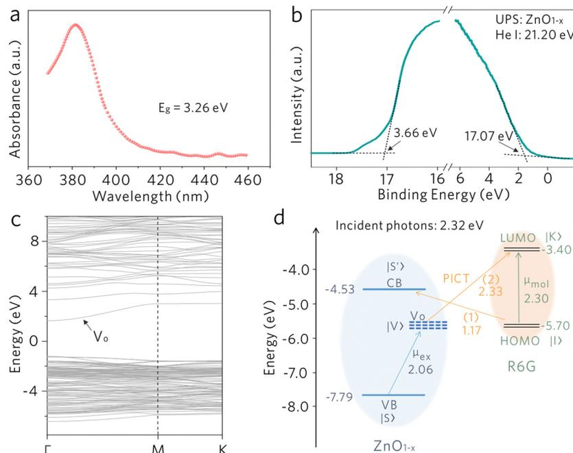
**Fig. 4** WGM cavity sensing mechanism: photoinduced charge transfer. (a) UV-vis spectrum of  $\text{ZnO}_{1-x}$ . (b) UPS spectrum of  $\text{ZnO}_{1-x}$ . (c) DFT calculations of the electronic band structure of  $\text{ZnO}_{1-x}$ ,  $V_o$  represent the oxygen-vacancy-associated defect level. (d) Energy level diagram of the R6G molecule on  $\text{ZnO}_{1-x}$  under the excitation of 532 nm (2.32 eV).
