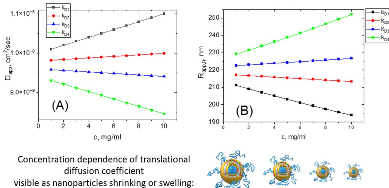
Fig. 7 The example of concentration dependence of apparent translational diffusion coefficient for different  $k_D$  values (A); the concentration dependence of apparent hydrodynamic radii calculated from  $D_t$  (B).
