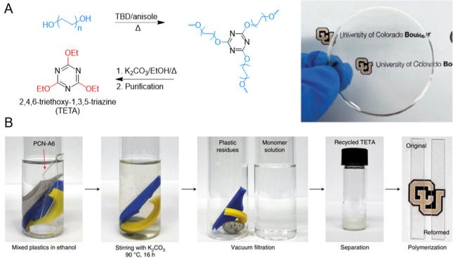
Fig. 14 (A) Depolymerization and synthesis of polycyanurate network polymers. (B) Polycyanurates can be depolymerized in the presence of ethanol and K<sub>2</sub>CO<sub>3</sub> added as a catalyst. Reproduced in part with permission from ref. 40. Copyright 2022 Nature Chem.
