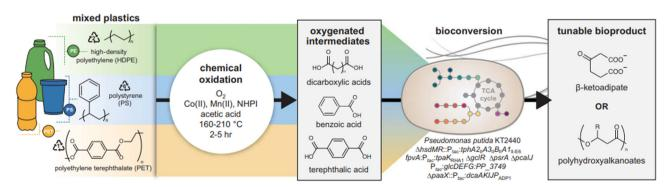
Fig. 9 Upcycling of mixed plastic waste through tandem chemical oxidation and bioconversion. Metal-promoted autoxidation simultaneously deconstructs multiple polymers, generating a mixture of oxygenated intermediates that are advantageous substrates for bioconversion. An engineered *P. putida* strain funnels the heterogeneous mixture of oxygenates into a single target product. Reproduced with permission from ref. 25. Copyright 2022 *Science*.
