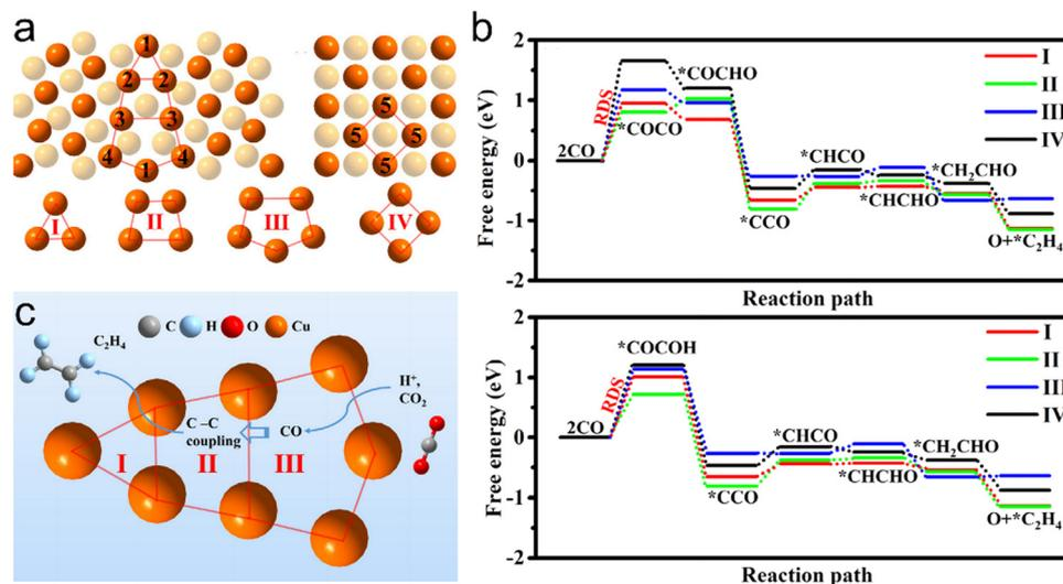
Fig. 3 (a) Cu atom structures of R5(021)/[100]GB and (100) facets, (b) the reaction pathways from CO<sub>2</sub> to C<sub>2</sub>H<sub>4</sub> based on (top) C–C coupling via \*COCO as an intermediate and (bottom) C–C coupling via \*COCO as an intermediate. (c) Diagram of the cascade reaction of C<sub>2</sub>H<sub>4</sub> between different sites on a GB surface. Reproduction with permission from ref. 93, Copyright 2022, Elsevier.
