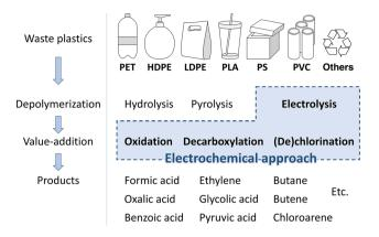
**Scheme 1** A schematic chart of the electrochemical upcycling of plastic waste.
