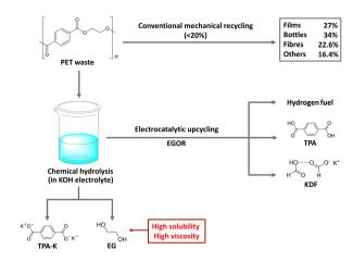
Fig. 5 Electrocatalytic PET upcycling to commodity chemicals and H<sub>2</sub> fuel. Reproduced with permission from ref. 51. Copyright 2021 Springer Nature.
