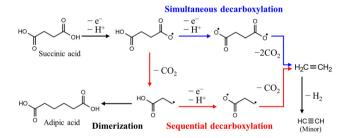
Fig. 10 Anodic decarboxylation pathways of succinic acid produced by the depolymerization of PE. Reproduced with permission form ref. 27. Copyright 2021 ACS publications.
