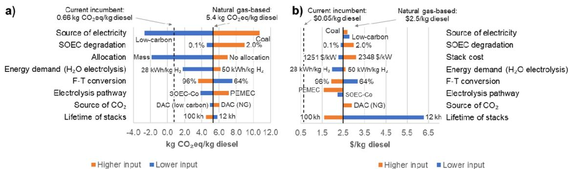
**Fig. 6** Parameter sensitivities to net CO<sub>2</sub> emissions from the base case for (a) LCA and (b) Economic analysis. The base case scenario is related to SOEC-W, natural gas-based electricity, CO<sub>2</sub>, heat, and steam, SOEC degradation of 0.5%/1000 h, F–T conversion of 80%, and system expansion *via* substitution. SOEC-W: SOEC water electrolysis, F–T: Fischer–Tropsch. The allocation methods (mass and no allocation) are applied to co-products O<sub>2</sub> and fuels.
