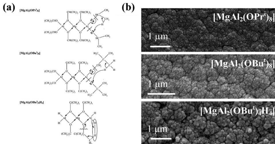
Fig. 16 (a) Proposed decomposition methods and (b) scanning electron microscopy surface images for precursors (top to bottom)  $[\text{MgAl}_2(\text{O}^i\text{Pr})_8]$ ,  $[\text{MgAl}_2(\text{O}^t\text{Pr})_8]$ ,  $[\text{MgAl}_2(\text{O}^i\text{Pr})_8]$ . Reproduced with permission from ref. 204 copyright 2004, American Chemical Society.
