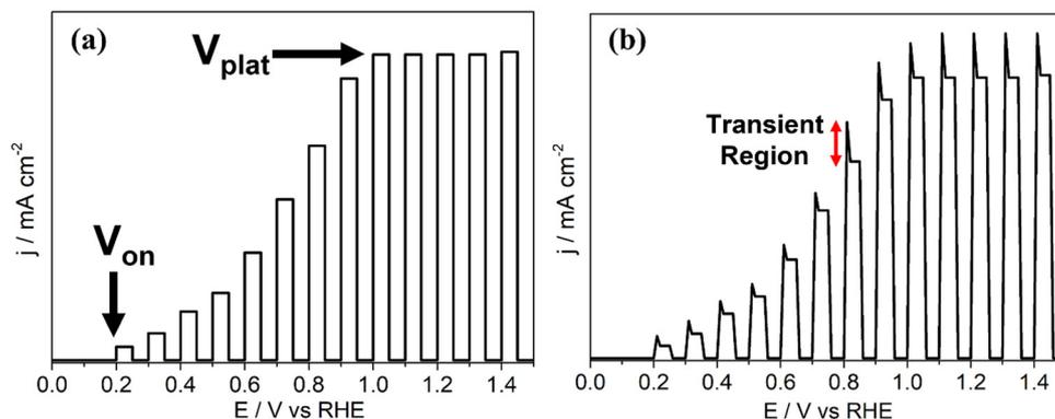
Fig. 6 Photocurrent density ( $j$ - $V$ ) graphs for example systems under chopped light showing (a) onset potential,  $V_{\text{on}}$ , and plateau potential,  $V_{\text{plat}}$ , (b) photocurrent transients.
