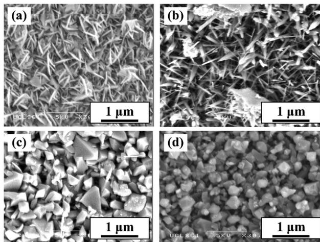
Fig. 17 Scanning electron micrographs of  $\text{TiO}_2$  grown on steel substrate by AACVD use carrier solvent of (a) ethanol, (b) methanol, (c) 10% methanol and 90% ethanol, (d) 25% methanol and 75% ethanol. Reproduced with permission from ref. 217 copyright 2012, Wiley-VCH.
