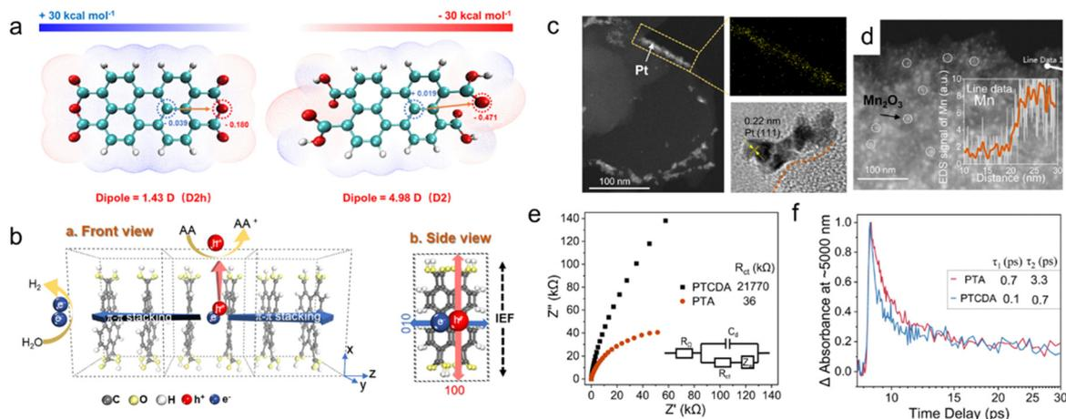
**Fig. 3** (a) Molecular dipole calculations. The dipole moment of PTCDA (left) and PTA (right) based molecular electrostatic potential. (b) Schematic diagram of IEF in PTA cell. ADF-STEM photodeposition on PTA with (c) Pt and high resolution and mapping, (d)  $\text{Mn}_2\text{O}_3$  (inset: Mn element liner scan). (e) impedance and (f) transient absorption decay kinetics at  $\sim 5000$  nm of PTCDA and PTA. Reproduced with permission from ref. 45 (Copyright 2022, Springer Nature).
