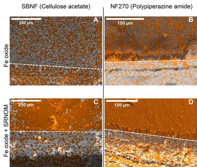
**Fig. 3** Elemental maps obtained by energy dispersive X-ray (EDX) analysis, showing iron-rich regions (in orange) overlaid on SEM micrographs of the cross-section and active layer of membranes (tilted 30–60°). Results shown for membranes fouled with: Fe oxide + CaCl<sub>2</sub> (A and B for SBNF and NF270, respectively); Fe oxide + SRNOM + CaCl<sub>2</sub> (C and D for SBNF and NF270, respectively). White dashed lines indicate the approximate location of the foulant-active layer interface.
