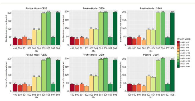
Fig. 2 The number of compounds that pass the QC across multiple collision energies in positive mode. Negative data is given in Fig. S3.†
