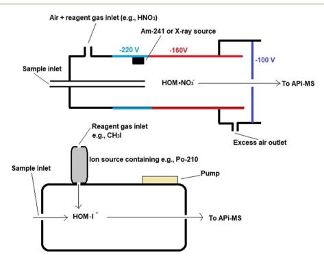
Fig. 2 Schematic structure of an Eisele-type ion source, reproduced from ref. 137 with permission from National Academy of Sciences, copyright 2014. An IMR ion source, reproduced from ref. 139 with permission from Copernicus Publications, copyright 2011.
