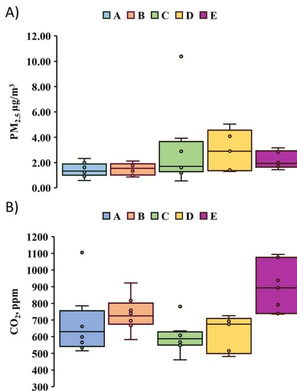
Fig. 6 Effect of MV (residence A–D) and NV (residence E) on indoor  $\text{PM}_{2.5}$  (A) and  $\text{CO}_2$  (B) concentration.
