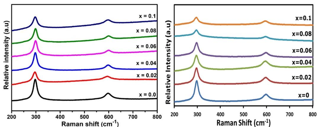
Fig. 8 Raman spectra of (lhs)  $\text{Ga}_x\text{Cd}_{1-x}\text{S}_{1+0.5x}$ , where  $x = 0, 0.02, 0.04, 0.06, 0.08$  and  $0.1$  and (rhs)  $\text{In}_x\text{Cd}_{1-x}\text{S}_{1+0.5x}$ , where  $x = 0, 0.02, 0.04, 0.06, 0.08$  and  $0.1$ .
