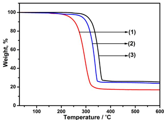
Fig. 1 Thermogravimetric analysis (TGA) profiles of (1) [Ga(DTC)<sub>3</sub>] (expected for Ga<sub>2</sub>S<sub>3</sub>; 22.9%), (2) [Cd(DTC)<sub>2</sub>] (expected for CdS; 25.5%) and (3) [In(DTC)<sub>3</sub>] (expected for In<sub>2</sub>S<sub>3</sub>; 29.1%).
