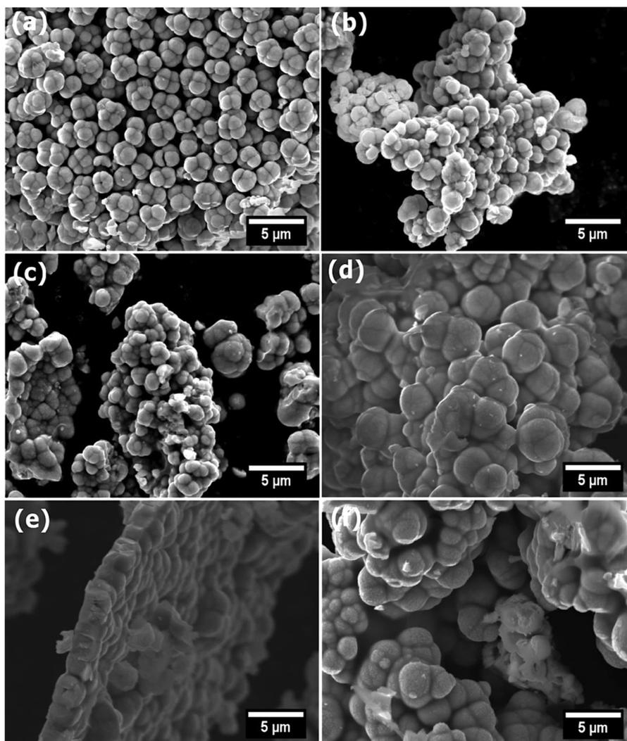
Fig. 3 Secondary electron SEM images (10 keV) of doped and undoped samples of  $\text{Ga}_x\text{Cd}_{1-x}\text{S}_{1+0.5x}$ ,  $x = 0$  (a),  $x = 0.02$  (b),  $x = 0.04$  (c),  $x = 0.06$  (d),  $x = 0.08$  (e) and  $x = 0.10$  (f).
