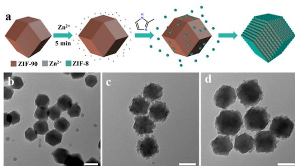
**Fig. 6** (a) Schematic illustration of the synthesis of ZIF-90@ZIF-8-B. (b–d) TEM images of the intermediate sample collected during the synthesis of ZIF-90@ZIF-8-B at different reaction times of 2 min, 5 min and 20 min. The scale bar is 100 nm.
