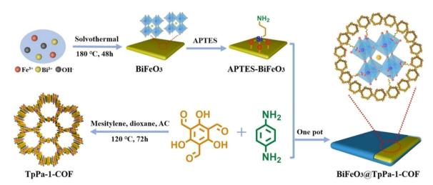
Fig. 18 Schematic illustration for fabricating a BiFeO<sub>3</sub>@TpPa-1-COF core-shell Z-scheme heterojunction hybrid. Adapted with permission, copyright, 2022, Wiley-VCH. 123
