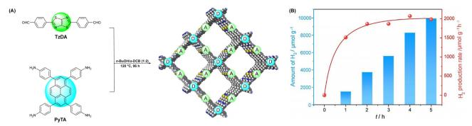
Fig. 4 (A) Schematic diagram of the fabrication of PyTz-COF. (B) Amount and rate of the hydrogen production of PyTz-COF. Reprinted with permission, copyright, 2021, Wiley-VCH.54
