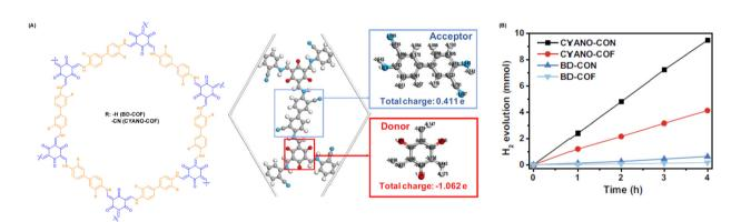
Fig. 7 (A) Structure diagram and charge distribution of CYANO-COF. (B) Time course of the photocatalytic H<sub>2</sub> evolution performance of different COFs and CONs. Reprinted with permission, copyright, 2022, Nature Publishing Group. 69
