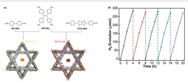
Fig. 3 (A) Schematic description showing the fabrication of PEBP-COF and PETZ-COF. (B) Testing the cycling stability of PETZ-COF hydrogen precipitation for more than 20 h. Reprinted with permission, copyright, 2022, Royal Society of Chemistry.<sup>53</sup>
