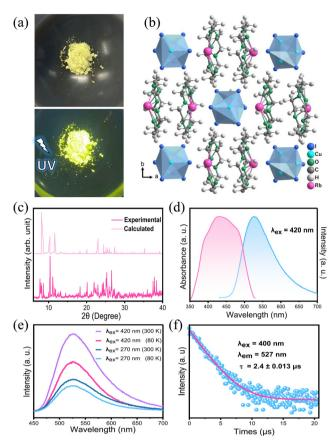
Fig. 1 (a) Images of RCCI powder under ambient light and UV irradiation (365 nm). (b) Crystal structure of [Rb(18-crown-6)]<sub>2</sub>Cu<sub>4</sub>I<sub>6</sub>·acetone, acetone is omitted for clarity. (c) PXRD pattern of RCCI-acetone. (d) Absorption and emission spectra of RCCI imaging screens. (e) Emission spectra of RCCI imaging screens at different excitation wavelengths (270 and 420 nm) and different temperatures (80 and 300 K). (f) Emission decay curves of RCCI imaging screens.
