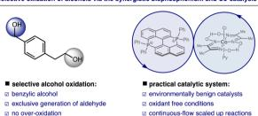
Fig. 1 Photocatalytic selective oxidation of benzylic alcohols via synergistic bisphosphonium and cobalt catalysis.
