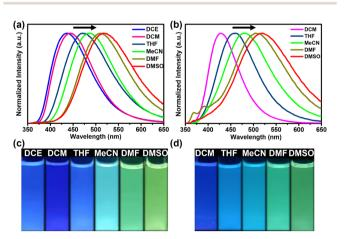
Fig. 4 The normalized fluorescence emission spectra of (a)  $[Ag_3(1)_2](PF_6)_3$ and (b)  $[Au_3(\mathbf{1})_2](PF_6)_3$  in various solvents ( $\lambda_{ex} = 330$  nm,  $c = 10^{-5}$  M, and T =298 K). Photographs of (c)  $[Ag_3(\mathbf{1})_2](PF_6)_3$  and (d)  $[Au_3(\mathbf{1})_2](PF_6)_3$  in various solvents under UV light.
