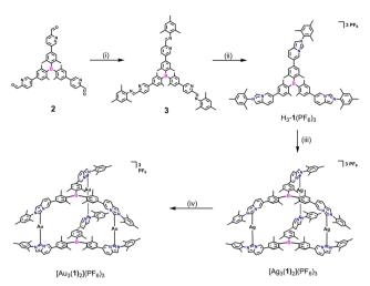
Scheme 1 Synthesis of the triarylborane-bridged NHC precursor H<sub>3</sub>-1(PF<sub>6</sub>)<sub>3</sub> and trinuclear hexacarbene complexes. (i) 2,4,6-Trimethylaniline, CH<sub>3</sub>COOH, CHCl<sub>3</sub>/EtOH, reflux; (ii) (a) paraformaldehyde, HCl, 25 °C; (b) NH<sub>4</sub>PF<sub>6</sub>, MeOH, 25 °C, yield 51%; (iii) Ag<sub>2</sub>O, CH<sub>3</sub>CN, 55 °C, yield 96%; (iv) AuCl(THT), CH<sub>3</sub>CN, 25 °C, yield 83%.
