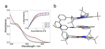
Fig. 2 (a) UV/Vis absorbance changes of  $\bf 1$  at 298 K (c = 0.05 mM in  $CH_3CN)$  upon the progressive addition of **2**. Inset: intensity changes in UV/ Vis absorbance at 510 nm, 525 nm, and 540 nm. The solid lines were obtained via a Matlab-based global analysis program. (b) Optimized structure of the host–guest complex  $1 \supset 2$  on the basis of DFT calculations.
