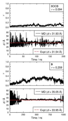
**Fig. 6** Translational order parameters,  $\tau$ , and layer spacings, d, from the MD simulations of 8OCB (top) and **9** (bottom). The average MD values given in the insets were determined over times 60–200 ns and 200–1000 ns for 8OCB and **9**, respectively, once the phase had formed and was relatively stable. The experimental values of d are given for the closest temperatures at which SAXS data were recorded (56.74 and 61.69 °C, respectively).
