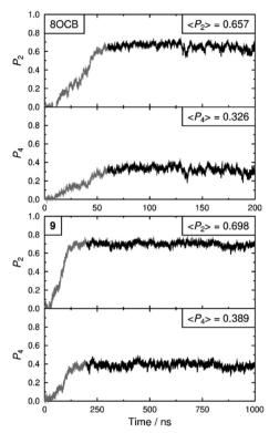
Fig. 5 Orientational order parameters,  $P_2$  and  $P_4$ , from the MD simulations of 8OCB (top) and 9 (bottom) vs. time. The average values given in the insets were determined over the region of each simulation represented by the heavier lines (60-200 ns and 200-1000 ns, respectively).
