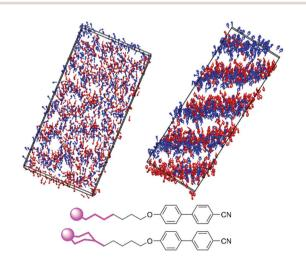
Fig. 10 Snapshots of the simulations of 8OCB at 75 ns (left) and 9 at 646 ns (right) showing the terminal alkyl carbon atoms from C<sub>4</sub> onwards, as shown in bold on the structures (bottom); the terminal carbon atoms are represented by spheres to assist orientation. Up and down molecules are coloured red and blue, respectively, and the simulation boxes are oriented with the laver normal vector vertical.
