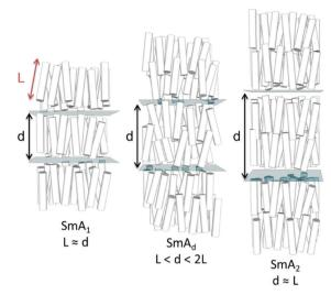
Fig. 1 Cartoon depictions of the sub types of the smectic A phase: monolayer (SmA $_1$ ), interdigitated (SmA $_d$ ) and bilayer (SmA $_2$ ). The molecules are indicated as cylinders with an aspect ratio of 10, the molecular length (L) and layer spacing (d) are indicated. The layers are shown as transparent planes, however in reality they are diffuse and disordered rather than being well defined.
