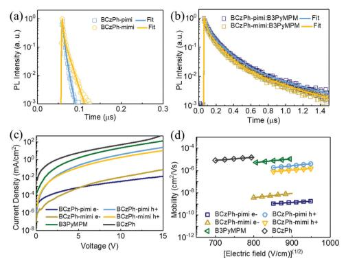
Fig. 5 (a) PL decay profiles of (a) bare BCzPh-pimi and BCzPh-mimi films and (b) BCzPh-pimi/B3PyMPM and BCzPh-mimi/B3PyMPM blended films. (c) Current densities of hole and electron only devices. (d) Hole and electron mobilities of each material
