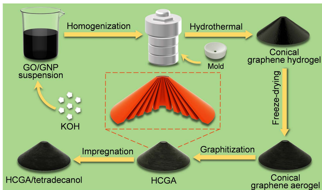
Fig. 1 Schematic illustrating the fabrication process of conical HCGA skeleton and its thermally conductive tetradecanol phase change composite.
