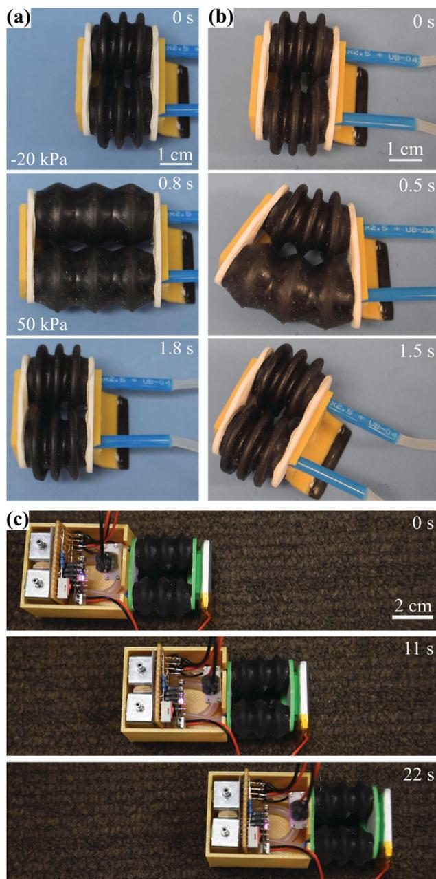
Fig. 6 Soft pneumatic locomotion robots. (a) Tethered robot forward motion steps, alternating between  $-20$  kPa and  $50$  kPa. (b) Tethered robot turning motion steps. (c) Untethered crawling traversing carpet.
