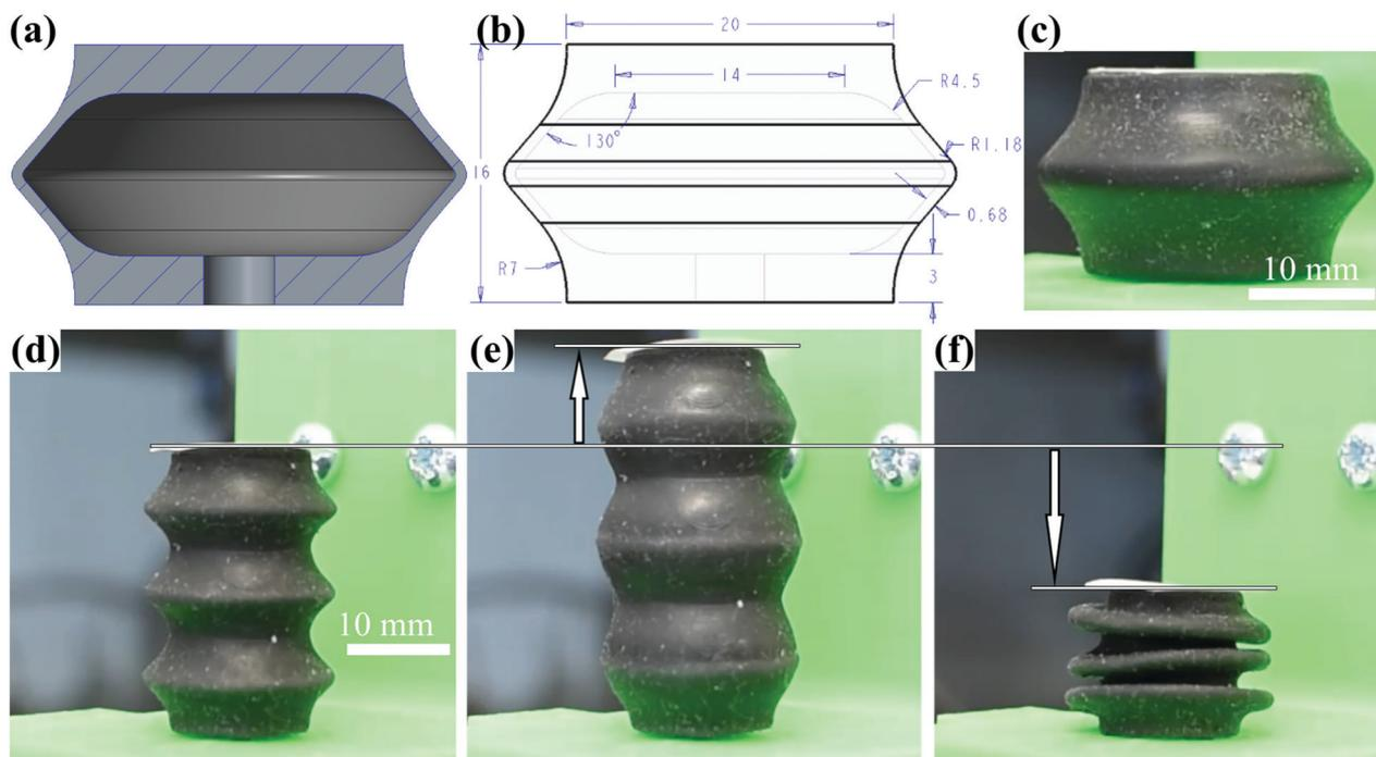
**Fig. 1** LSOMMA diagrams and photos. (a) Cross-sectional side view of a 1C LSOMMA. (b) Side view of a 1C 20 mm LSOMMA with dimensions labelled. (c) 1C 20 mm LSOMMA at rest. (d) 3C 14 mm LSOMMA at rest. (e) 3C 14 mm LSOMMA with 75 kPa applied. (f) 3C 14 mm LSOMMA with  $-25$  kPa applied.
