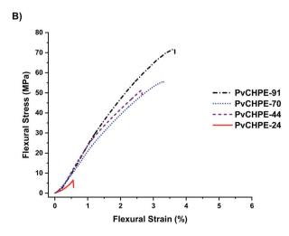
Fig. 3 Thermal and mechanical data for PvCHPE samples (Table 2). (A) DSC data shows the increase in  $T_g$  with molar mass. (B) Representative bending stress–strain data for PvCHPE samples (DMA; 3-point bend method, 0.1% s min<sup>-1</sup>, 25 °C).
