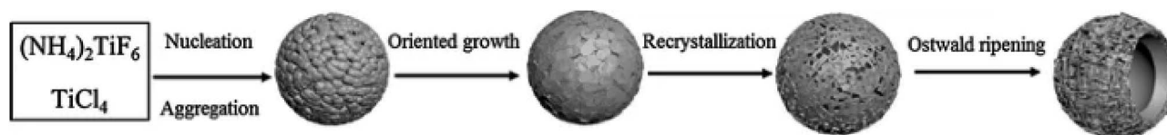
Fig. 6 Schematic illustration of the probable formation mechanism of hollow porous TiO 2 microspheres. 97
