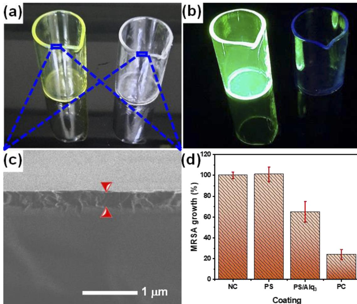
Fig. 9 PS/Alq<sub>3</sub> as an antibacterial composite: (a) and (b) 10 ml glass beaker coated with a PS polymer and a PS/Alq<sub>3</sub> composite under visible light and UV irradiation ( $\lambda = 385$  nm), respectively; (c) SEM image of the cross-sections of the coated beakers; and (d) histogram demonstrating the MRSA growth ratio after incubation for 24 h in the NC, PS, PS/Alq<sub>3</sub> (2% Alq<sub>3</sub>), and PC (5  $\mu\text{g ml}^{-1}$ ) group beakers.
