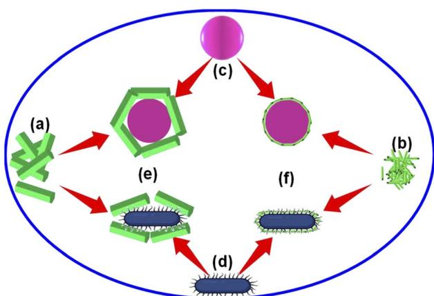
Fig. 7 Schematic diagram presenting the antimicrobial activity mechanism of the Alq<sub>3</sub> samples: (a) Alq<sub>3</sub> as rec, (b) Alq<sub>3</sub> NPs, (c) coccus bacteria, (d) bacillus bacteria, (e) cross-section of bacteria surrounded by the microparticles of the sample Alq<sub>3</sub> as rec and (f) cross-section of bacteria surrounded by the nanoparticles of the sample Alq<sub>3</sub> NPs.
