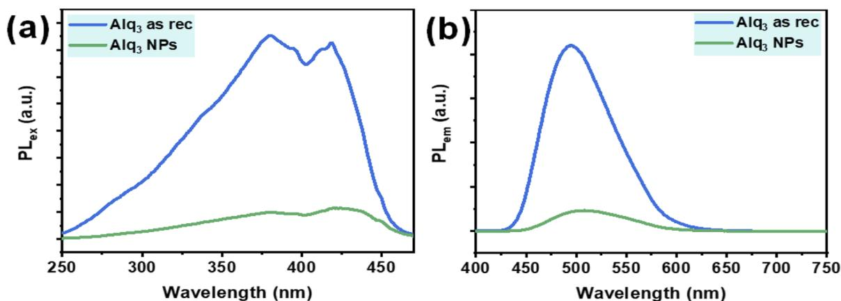
Fig. 5 PL spectra of the Alq<sub>3</sub> as rec and Alq<sub>3</sub> NP samples: (a) excitation spectra ( $\lambda_{em} = 500$  nm) and (b) emission spectra ( $\lambda_{ex} = 380$  nm).
