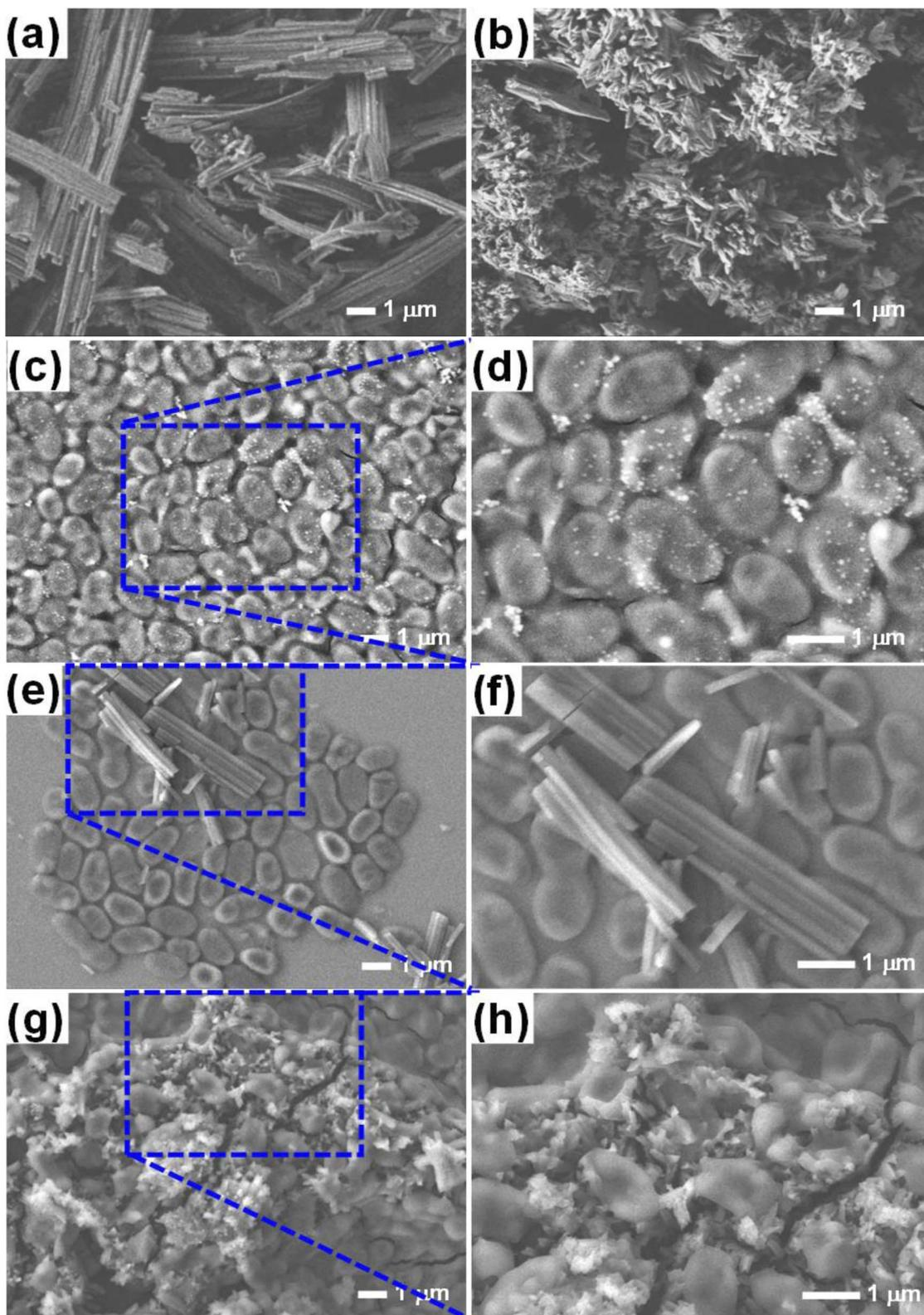
Fig. 8 SEM images of (a) Alq<sub>3</sub> as rec, (b) Alq<sub>3</sub> NP, (c and d) MRSA growth in MHB without treatment with Alq<sub>3</sub>, (e and f) MRSA growth in MHB including 20 μg ml<sup>-1</sup> of Alq<sub>3</sub> as rec, and (g and h) MRSA growth in MHB including 20 μg ml<sup>-1</sup> of Alq<sub>3</sub> NPs.
