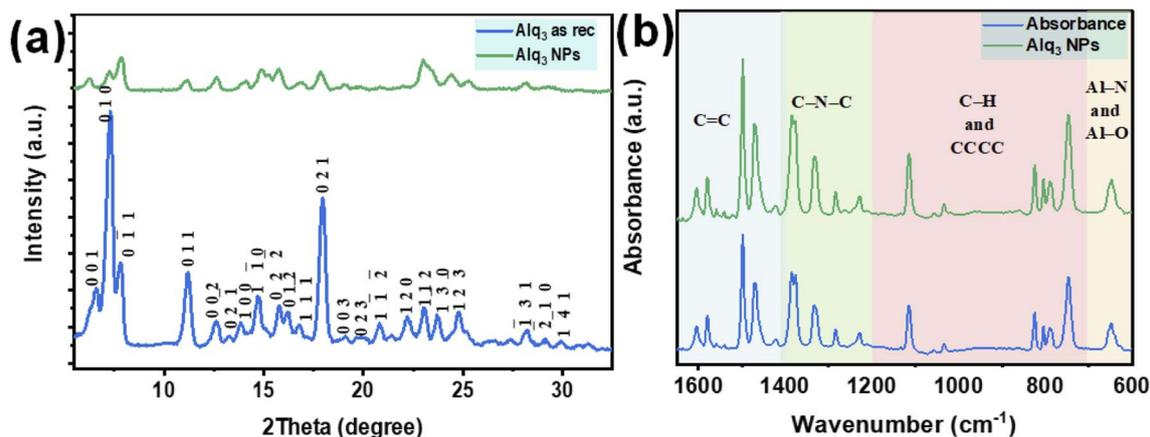
Fig. 4 (a) XRPD patterns and (b) FTIR spectra of the Alq<sub>3</sub> as rec and Alq<sub>3</sub> NP samples' powders.
