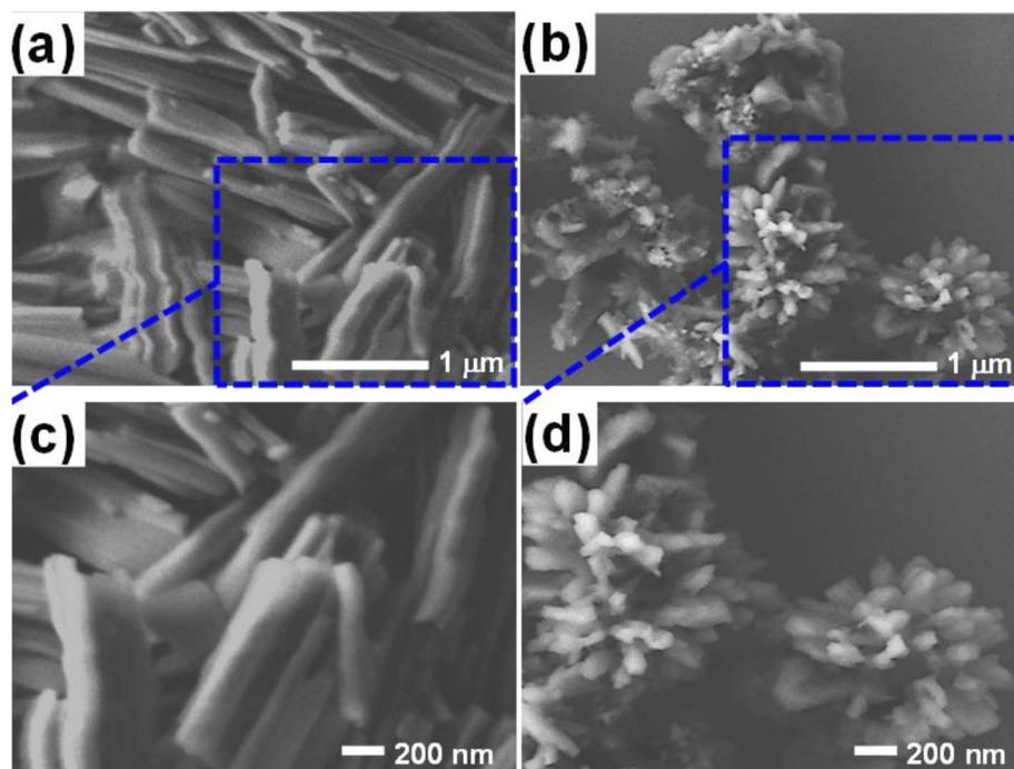
Fig. 3 SEM images of the Alq<sub>3</sub> samples: (a) and (b) images of Alq<sub>3</sub> as rec and Alq<sub>3</sub> NP samples, respectively; (c) and (d) their images at a higher magnification.
