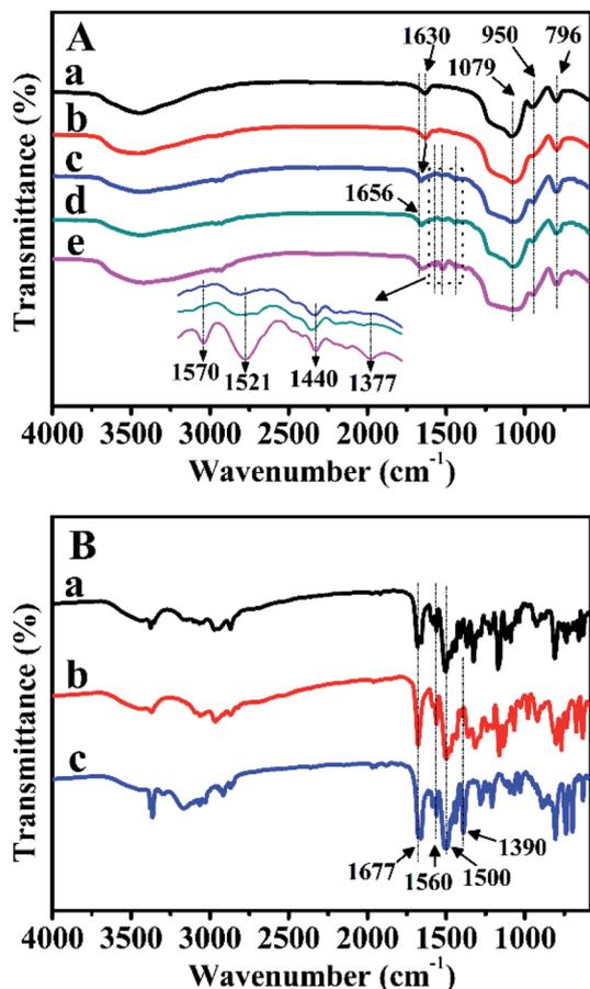
Fig. 7 FT-IR spectra of (A) BMMs-based samples. (a) Pure mesoporous materials, (b) Zn-modified samples, (c)  $Z_1$ -immobilized samples, (d)  $Z_2$ -immobilized samples, and (e)  $Z_3$ -immobilized samples, in which the molar ratios of Z/Zn for all samples were around 1 : 1. (B-a)  $Z_1$ , (B-b)  $Z_2$ , and (B-c)  $Z_3$ .
