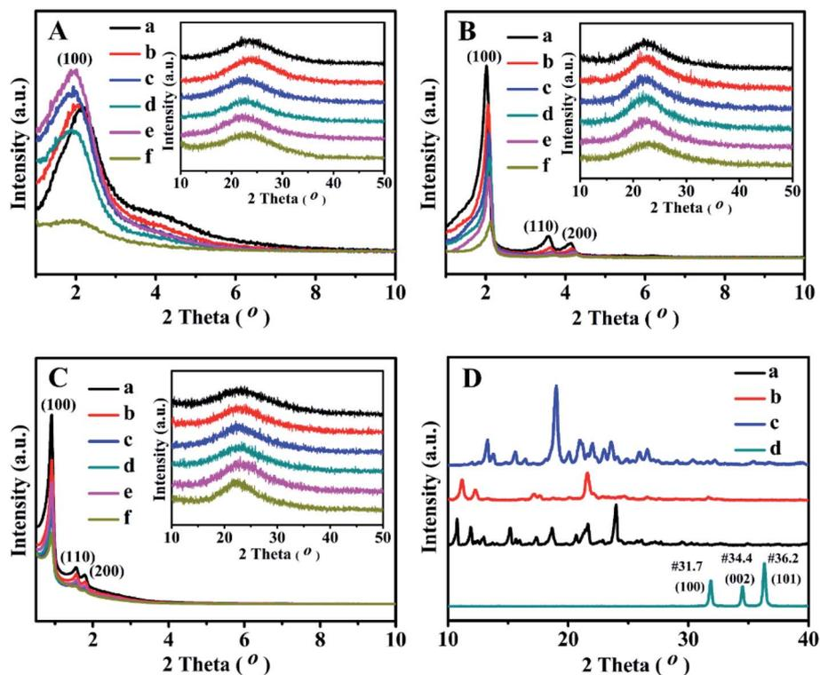
Fig. 3 Small and wide (inset) angle XRD patterns of (A) BMMs-, (B) MCM-41-, and (C) SBA-15-based samples. (a) Pure mesoporous materials, (b) Zn-modified samples, (c)  $Z_1$ -immobilized samples, (d)  $Z_2$ -immobilized samples, (e)  $Z_3$ -immobilized samples, and (f) 3<sup>rd</sup> recycled  $Z_2$ -immobilized samples, in which the molar ratios of Z/Zn for all samples were around 1 : 1. (D) Wide-angle XRD patterns of synthesized (a)  $Z_1$ , (b)  $Z_2$ , (c)  $Z_3$ , and (d) ZnO.
