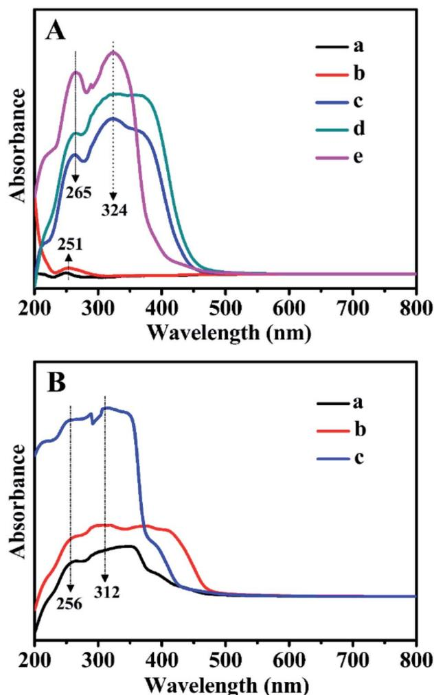
Fig. 8 UV-Vis DR spectra of (A) BMMs-based samples. (a) Pure mesoporous materials, (b) Zn-modified samples, (c)  $Z_1$ -immobilized samples, (d)  $Z_2$ -immobilized samples, and (e)  $Z_3$ -immobilized samples, in which the molar ratios of Z/Zn for all samples were around 1 : 1. (B-a)  $Z_1$ , (B-b)  $Z_2$ , and (B-c)  $Z_3$ .
