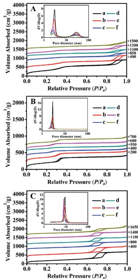
Fig. 4  $N_2$  adsorption-desorption isotherms and corresponding pore size distribution (inset) of (A) BMMs-, (B) MCM-41-, and (C) SBA-15-based samples. (a) Pure mesoporous materials, (b) Zn-modified samples, (c)  $Z_1$ -immobilized samples, (d)  $Z_2$ -immobilized samples, and (e)  $Z_3$ -immobilized samples, and (f) 3<sup>rd</sup> recycled  $Z_2$ -immobilized samples, in which the molar ratios of Z/Zn for all samples were around 1 : 1.
