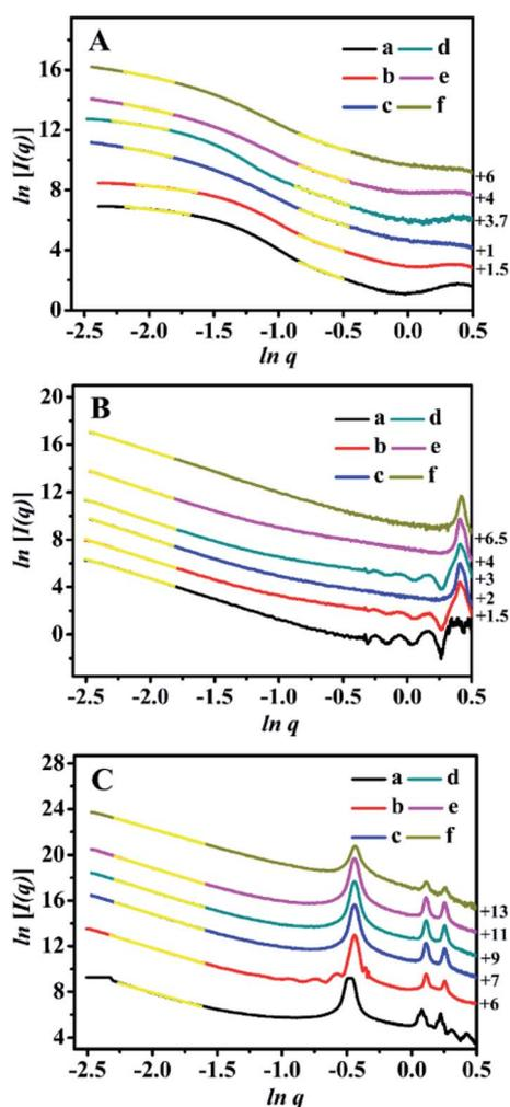
Fig. 1 Shifted scattering curves (offset values in left Y-axis) of (A) BMMs-, (B) MCM-41-, (C) SBA-15-based samples, (a) pure mesoporous materials, (b) Zn-modified samples, (c)  $Z_1$ -immobilized samples, (d)  $Z_2$ -immobilized samples, (e)  $Z_3$ -immobilized samples, and (f) 3<sup>rd</sup> recycled  $Z_2$ -immobilized samples. The molar ratios of Z/Zn for all samples were around 1 : 1.
