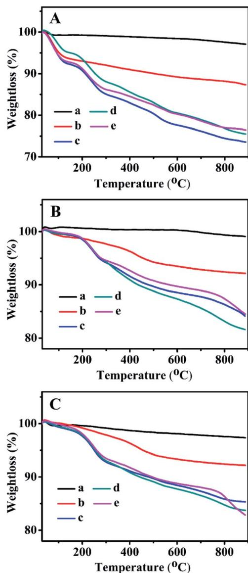
Fig. 6 TGA curves of (A) BMMs-, (B) MCM-41-, and (C) SBA-15-based samples. (a) Pure mesoporous materials, (b) Zn-modified samples, (c)  $Z_1$ -immobilized samples, (d)  $Z_2$ -immobilized samples, and (e)  $Z_3$ -immobilized samples, in which the molar ratios of Z/Zn for all samples were around 1 : 1.
