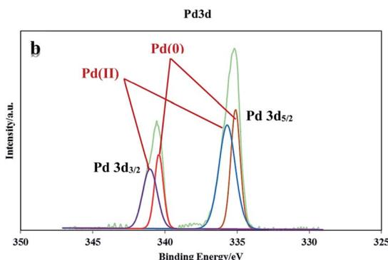
Fig. 6 XPS patterns of PAMAM  $G_0$ -Pd@ $\gamma$ -Fe<sub>2</sub>O<sub>3</sub>: overall elemental survey spectrum (a), and, Pd3d (b).
