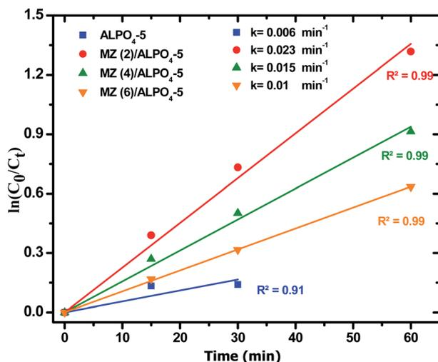
Fig. 10 First order plots of PNP degradation over prepared catalysts. Reaction conditions: the dosage of catalysts  $1.0 \text{ g l}^{-1}$ , initial PNP concentration of  $0.04 \text{ g l}^{-1}$  after 180 min irradiation time.
