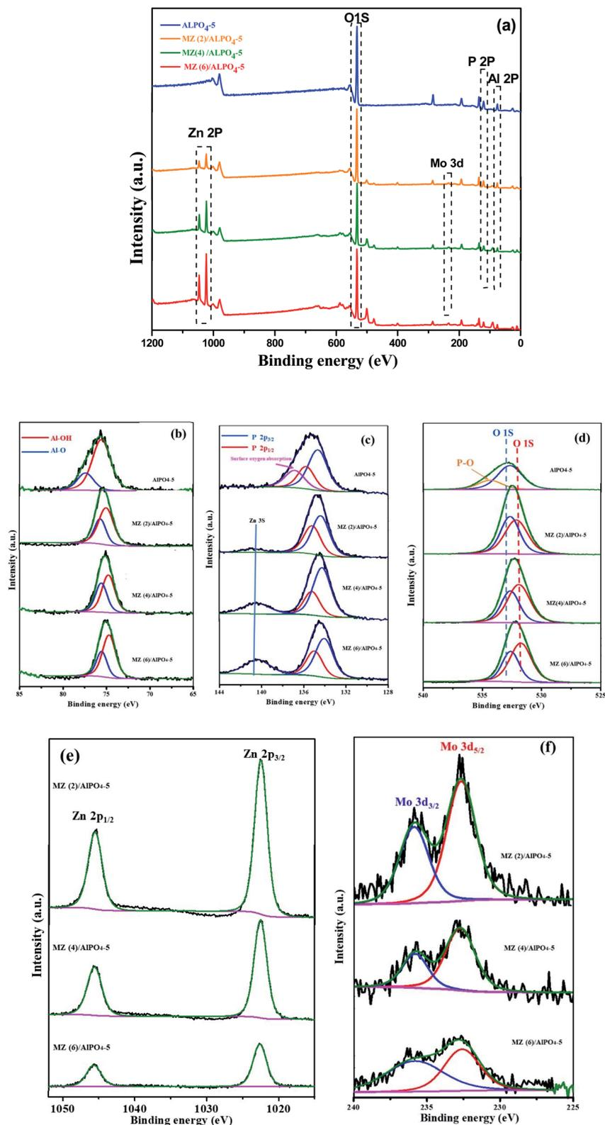
Fig. 5 XPS spectra of Mn/Zn (x)  $\text{AlPO}_4\text{-}5$ ,  $X = 0, 0.1, 0.2$  or  $0.3$  nanocomposites (a) survey of the samples, (b) Al, (c) P, (d) O, (e) Zn and (f) Mo spectra.
