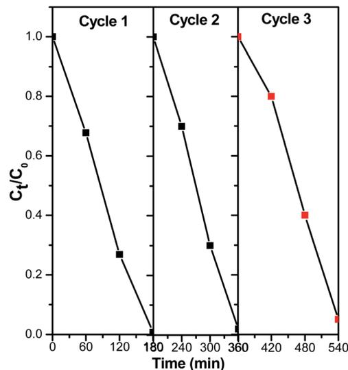
Fig. 11 Recycling performance of ZnMoO<sub>4</sub>/AlPO<sub>4</sub>-5 with MZ (2) for PNP degradation in an aqueous solution. Reaction conditions: the dosage of catalysts  $1.0 \text{ g l}^{-1}$ , initial PNP concentration of  $0.04 \text{ g l}^{-1}$  after 180 min irradiation time for each cycle.
