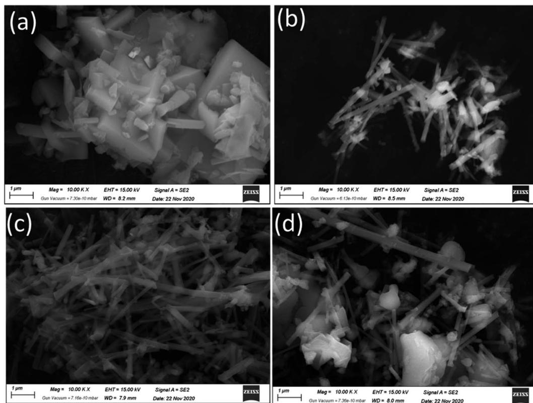
Fig. 4 FE-SEM images of the as-prepared (a)  $\text{AlPO}_4\text{-5}$  molecular sieves, and (b–d)/MZ (2, 4 and 6)  $\text{AlPO}_4\text{-5}$  nanocomposite.
