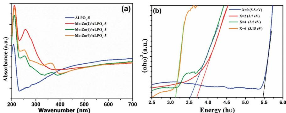
Fig. 6 UV-Vis diffuse reflectance spectra (a) and  $(\alpha h\nu)^2$  vs.  $h\nu$  curves (b) of  $\text{AlPO}_4\text{-5}$  molecular sieves, and MZ (2, 4 and 6)  $\text{AlPO}_4\text{-5}$  nanocomposites.
