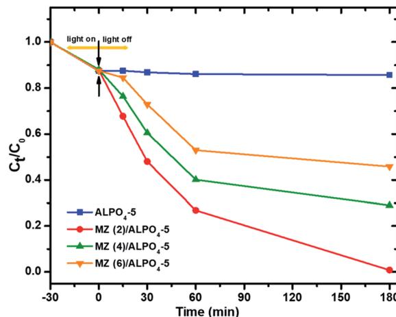
Fig. 9 Photocatalytic degradation of PNP over prepared catalysts. Reaction conditions: the dosage of catalysts  $1.0 \text{ g l}^{-1}$ , initial PNP concentration of  $0.04 \text{ g l}^{-1}$  after 180 min irradiation time.
