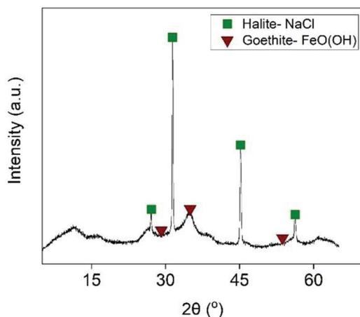
Fig. 10 X-ray diffractogram of the iron-rich precipitate.
