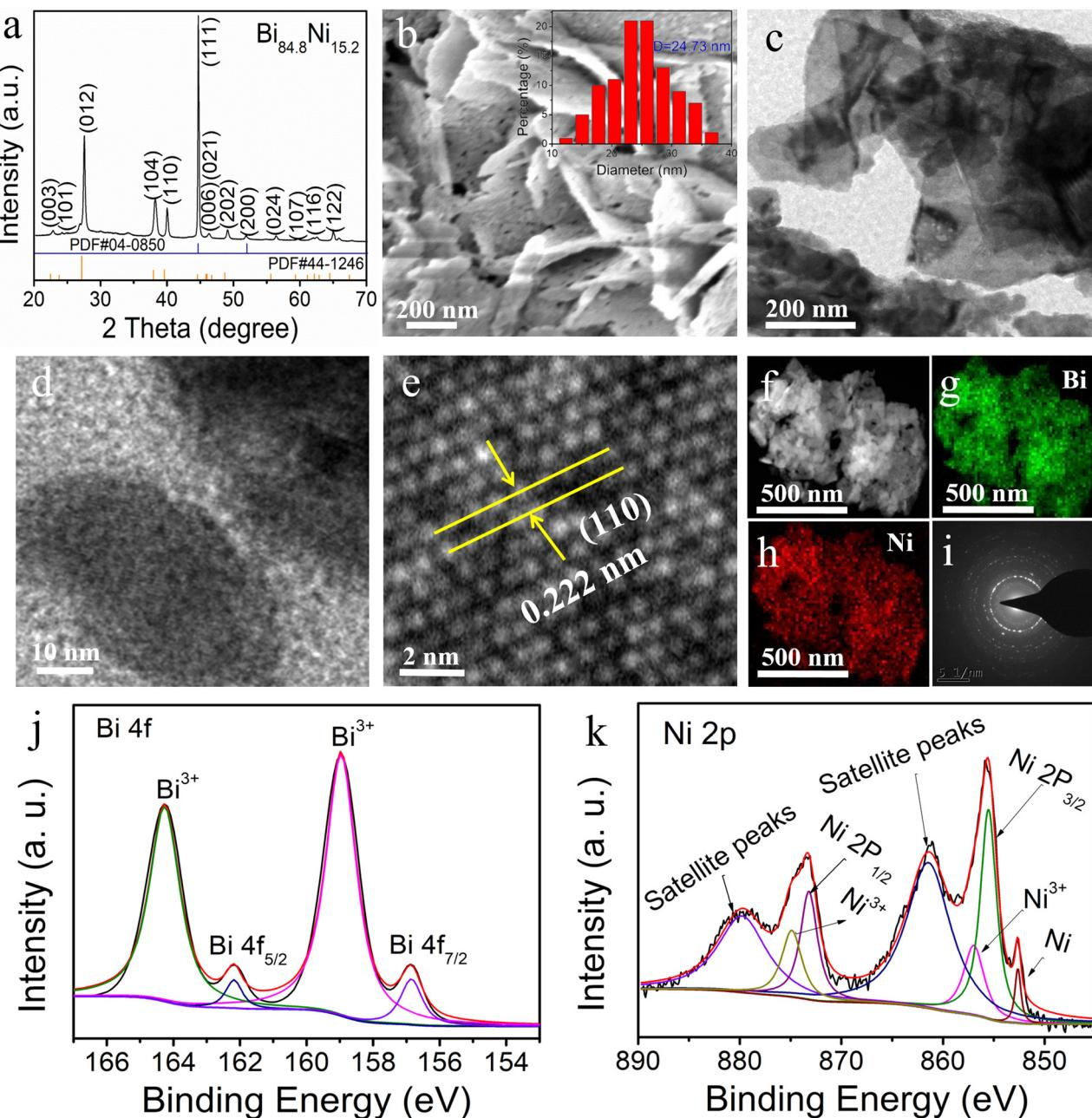
**Fig. 1** Characterizations of mesoporous Bi<sub>84.8</sub>Ni<sub>15.2</sub> alloy (a) XRD patterns; (b) SEM image; inset: pore-distribution image; (c and d) TEM images; (e) HRTEM image; (f) HAADF-STEM image; (g and h) EDS mapping images; (i) SAED pattern; (j) XPS spectrum of Bi 4f; (k) XPS spectrum of Ni 2p.
