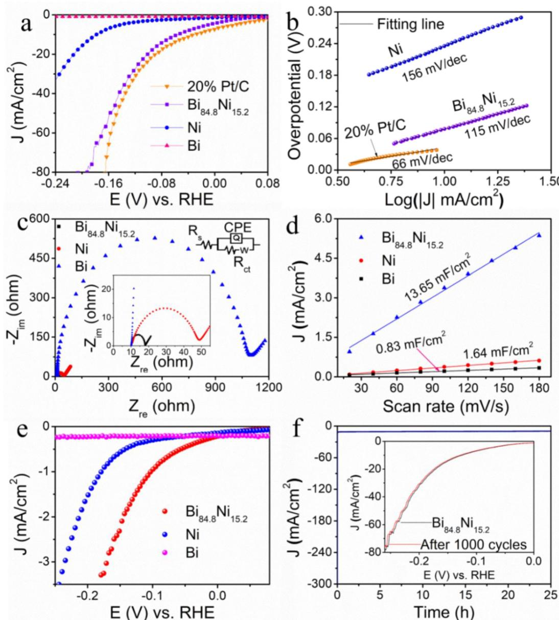
**Fig. 2** (a) Polarization curves of samples for HER in 1.0 M KOH; (b) Tafel plots; (c) Nyquist plots at  $-56$  mV vs. RHE. Inset shows the equivalent circuit; (d) capacitive current as a function of scan rate for the samples; (e) specific activity; (f)  $I-t$  test for  $\text{Bi}_{84.8}\text{Ni}_{15.2}$  alloy at  $-56$  mV vs. RHE; inset shows the polarization curves at  $5$  mV s<sup>-1</sup> before and after 1000 cycles of CV.
