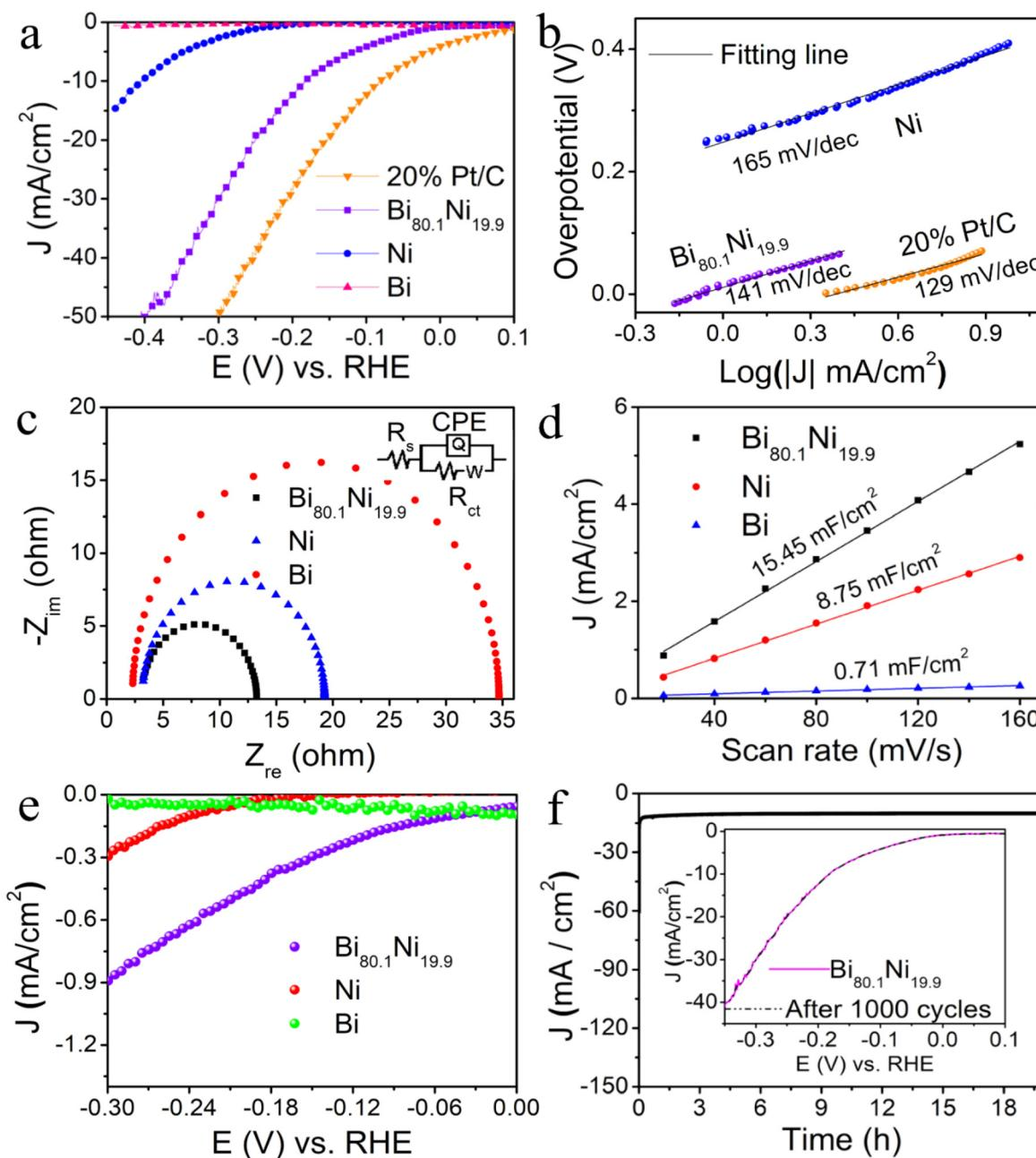
**Fig. 3** (a) Polarization curves for HER in 1.0 M PBS (pH 7.0); (b) Tafel plots; (c) Nyquist plots at  $-183$  mV vs. RHE. Inset shows the equivalent circuit; (d) capacitive current as a function of scan rate for the samples; (e) specific activity; (f)  $I$ - $t$  test for  $\text{Bi}_{80.1}\text{Ni}_{19.9}$  alloy at  $-183$  mV vs. RHE; inset shows the polarization curves at  $5\text{ mV s}^{-1}$  before and after 1000 cycles CV.
