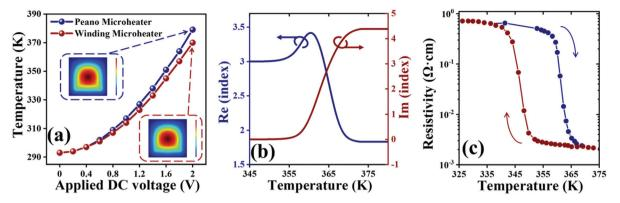
Fig. 4 (a) The relationships between the applied DC voltages and heating temperatures of the Peano-shaped microheater. The inserted images show the temperature distributions of the Peano-shaped microheater with a driving voltage of 2.0 volts. (b) Variation of the index of  $VO_2$  with different heating temperatures at a wavelength of 2.70  $\mu$ m. (c) Variation of the resistivity of  $VO_2$  with different heating temperatures.
