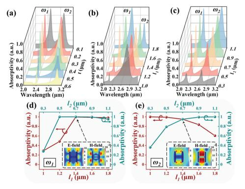
Fig. 2 Absorptivity of the H-shaped MPA with different (a)  $t_1$ , (b)  $l_2$ , and (c)  $l_2$  values, respectively. The relationships of the resonance intensities of the H-shaped MPA with different  $l_1$  and  $l_2$  values at (d)  $\omega_1$  and (e)  $\omega_2$  resonances, respectively. The inserted images show the corresponding E-field and H-field distributions under the conditions of  $l_1$  = 1.4  $\mu$ m and  $l_2$  = 0.7  $\mu$ m.
