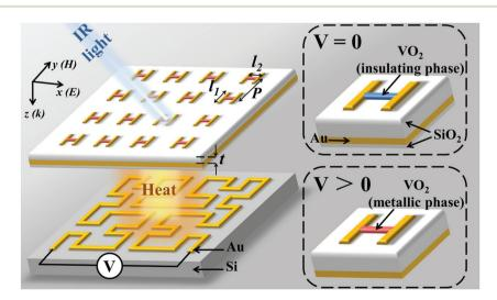
Fig. 1 Schematic drawing and tuning mechanism of MEMS-based MPA design. The periods of unit cells are kept as  $P = 2.3 \mu m$ .
