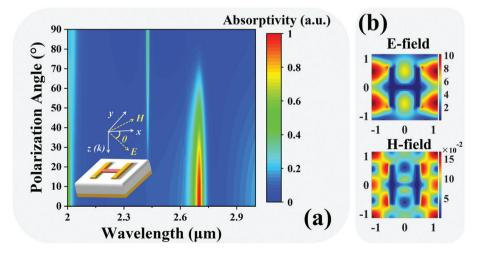
Fig. 3 (a) Absorptivity of the H-shaped MPA at different polarization angles. (b) The corresponding E-field and H-field distributions with a polarization angle of 90° at a wavelength of 2.40 µm.
