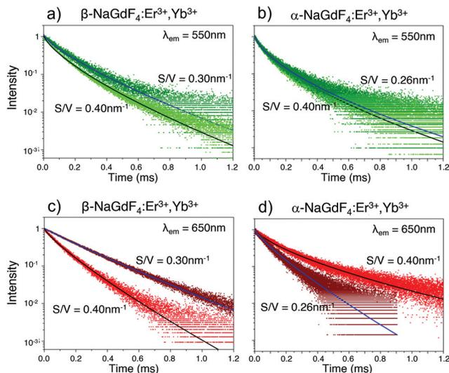
**Fig. 7** UC luminescence decay curves for (a), (c)  $\beta$ - and (b), (d)  $\alpha$ - $\text{NaGdF}_4$  UCNP of two different sizes ( $S/V$  as labeled in the figure) dispersed in toluene monitoring either the UCNP's green ( $\lambda_{\text{em}} = 550 \text{ nm}$ ) or red ( $\lambda_{\text{em}} = 650 \text{ nm}$ ) emission following 980 nm excitation. From these decay curves, respective excited state lifetimes have been determined using a Kohlrausch fitting function (solid lines).
