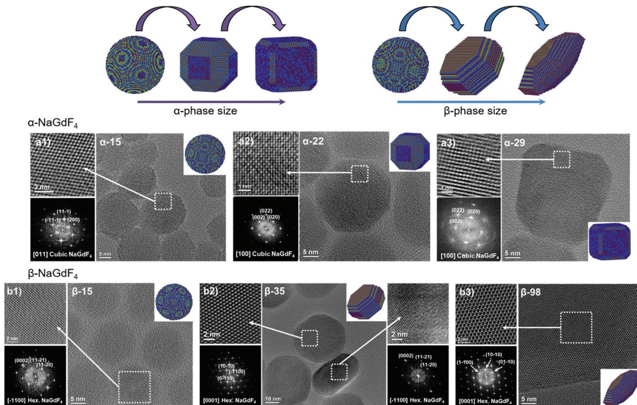
Fig. 2 HRTEM images, SAED patterns and morphological models of selected (a)  $\alpha$ - and (b)  $\beta$ - $\text{NaGdF}_4:\text{Er}^{3+}/\text{Yb}^{3+}$  UCNPs (additional data available in Fig. S2<sup>†</sup>).
