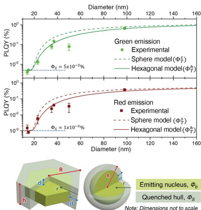
**Fig. 5**  $\beta$ - $\text{NaGdF}_4$  experimental PLQY data (green emission on top, red emission below) fitted to a simple nucleus/hull volumetric model assuming spherical (dashed lines) and hexagonal particles (full line). A scheme of the two shapes indicating the different parameters used for their definition is given below the graphs.
