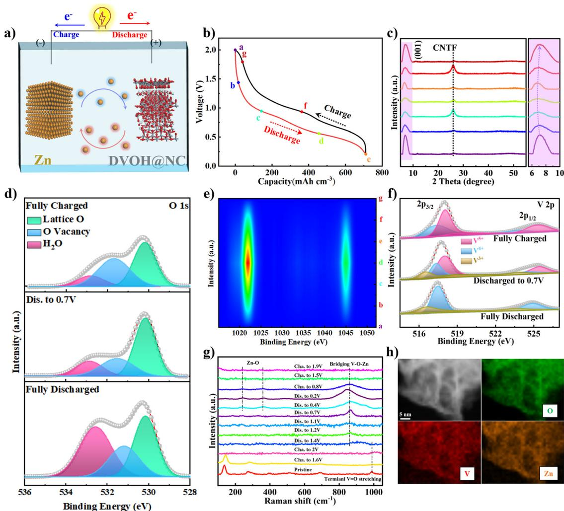
Fig. 5 (a) Schematic of the ion and electron transport behavior in the DVOH@NC@CNTF//Zn battery. (b and c) Various points in the second discharge/charge process for *ex situ* XRD tests. Fine XPS spectra of the material in different states of charge: (d) O 1s, (e) Zn 2p, and (f) V 2p. (g) *Ex situ* Raman spectra obtained during the charging/discharging processes. (h) TEM image of DVOH nanosheets and the corresponding elemental mappings of O, V, and Zn at the fully discharged state.
