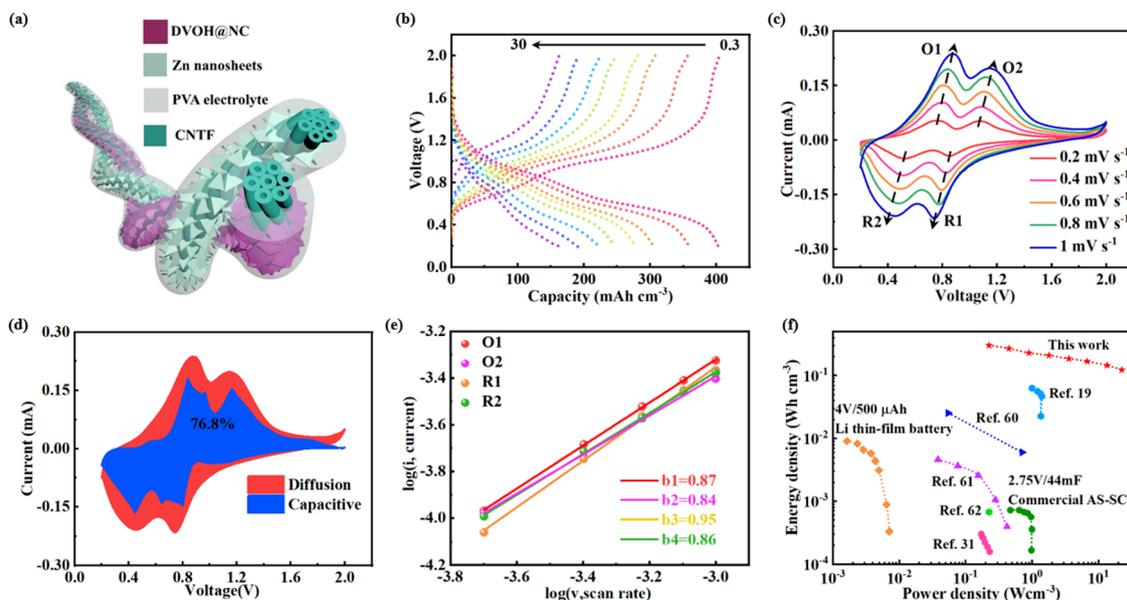
**Fig. 6** (a) Schematic configuration of FAZIBs. (b) GCD curves at various current densities of DVOH@NC@CNTF||Zn@CNTF FAZIBs. (c) CV of DVOH@NC@CNTF||Zn@CNTF FAZIBs at different scan rates. (d) Capacitive and diffusion contributions to charge storage of DVOH@NC@CNTF||Zn@CNTF FAZIBs at 1  $\text{mV s}^{-1}$ . (e) The calculated *b*-values from CV curves at different scan rates of DVOH@NC@CNTF||Zn@CNTF FAZIBs. (f) Ragone plot of our DVOH@NC@CNTF||Zn@CNTF FAZIBs and previously reported FAZIBs.
