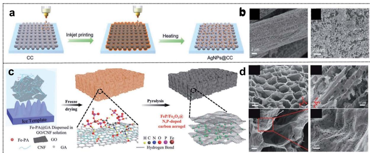
**Fig. 6** Foldable 3D electrode. (a) Schematic illustration of the fabrication process of AgNPs@CC. (b) SEM images of AgNPs@CC scaffolds. Reproduced from ref. 91. Copyright 2021, Wiley-VCH. (c) Schematic illustration of the fabrication process of FeP/Fe<sub>2</sub>O<sub>3</sub>@NPCA. (d) SEM images of FeP/Fe<sub>2</sub>O<sub>3</sub>@NPCA at different magnifications. Reproduced from ref. 92. Copyright 2020, Wiley-VCH.
