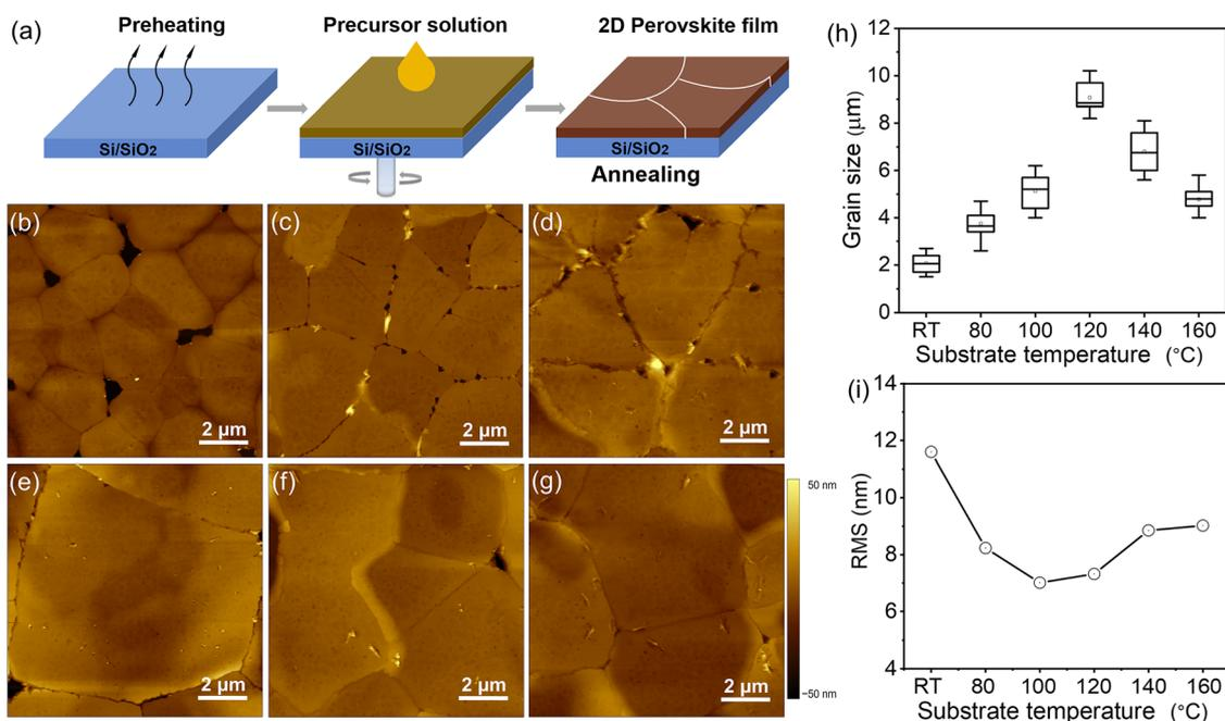
**Fig. 2** (a) Schematic diagram of the hot-casting process. AFM height images of thin  $(\text{TEA})_2\text{SnI}_4$  films processed at the substrate temperature of (b) RT, (c) 80 °C, (d) 100 °C, (e) 120 °C, (f) 140 °C and (g) 160 °C. (h) Grain size and (i) film root mean square roughness as a function of substrate temperature.
