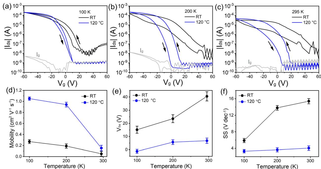
Fig. 5 Transfer characteristics measured at (a) 100 K, (b) 200 K, and (c) 295 K with  $L = 30 \mu\text{m}$ ,  $W = 1000 \mu\text{m}$ . The gray curves are the leakage currents ( $I_{\text{g}}$ ) between the source and gate electrodes in the 120 °C cast device. (d) Average hole charge carrier mobility, (e) threshold voltage and (f) subthreshold swing as a function of FET temperature. The error bars were calculated from 12 devices.
