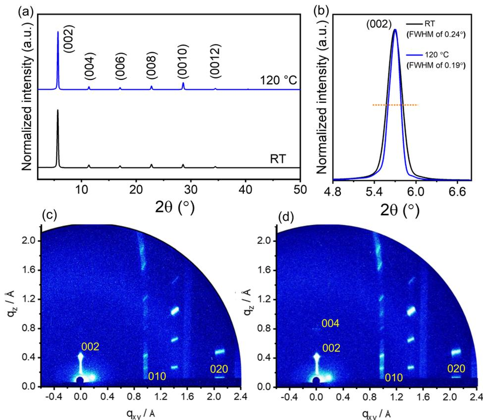
Fig. 3 (a) Out-of-plane XRD measured for (TEA)<sub>2</sub>SnI<sub>4</sub> thin films cast at RT and 120 °C. (b) FWHM analysis of the (002) peak. GIWAXS patterns for (TEA)<sub>2</sub>SnI<sub>4</sub> cast at (c) RT and (d) 120 °C (reflections are assigned by Miller indices).
