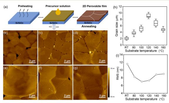
Fig. 2 (a) Schematic diagram of the hot-casting process. AFM height images of thin (TEA)<sub>2</sub>SnI<sub>4</sub> films processed at the substrate temperature of (b) RT, (c) 80 °C, (d) 100 °C, (e) 120 °C, (f) 140 °C and (g) 160 °C. (h) Grain size and (i) film root mean square roughness as a function of substrate temperature.
