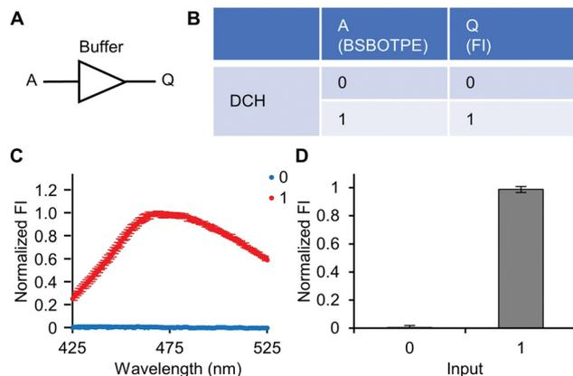
**Fig. 2** Buffer logic operation. (A) Symbol of logic gate. (B) Truth table. (C) The normalized fluorescence spectra of logic operation with different inputs. (D) Normalized FI at 471 nm. The concentrations of DCH and BSBOTPE used are 6  $\mu\text{M}$  and 141  $\mu\text{M}$ , respectively. Excitation wavelength was set at 350 nm.  $n = 3$ .
