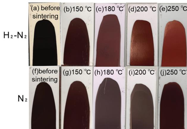
Fig. 7 Digital images of the surface of the sintered copper nanoparticle layers. (a) Before sintering, (b–e) sintered at various temperatures indicated in the image under 3%H<sub>2</sub>-N<sub>2</sub> gas flow, (f) before sintering, (g–j) sintered at various temperatures under nitrogen gas flow.
