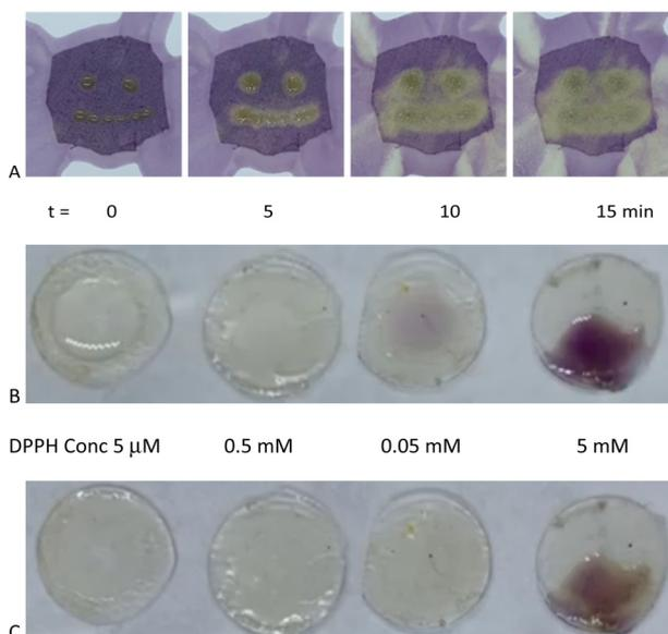
**Fig. 4** (A) **5P-17** spotted onto cotton fabric soaked with DPPH (purple, 5 mM) in IPA; time lapse over 5 minutes showing both antioxidant activity and diffusion of oil through the fabric. (B) From left to right, 5  $\mu$ M, 0.05 mM, 0.5 mM, and, 5 mM DPPH in IPA solution spotted onto **5E-75**  $t = 15$  s, (C)  $t = 90$  s.
