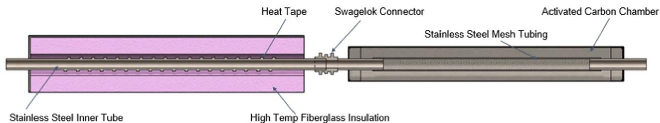
Fig. 2 Cross-sectional view of the thermodenuder used in the study, highlighting its different components. The temperature of the heating section was monitored *via* a K-type thermocouple placed at the mid-section surface of the sampling tube, providing feedback to an external temperature controller unit. The aerosol flow direction is from the left towards the denuder section to the right.
