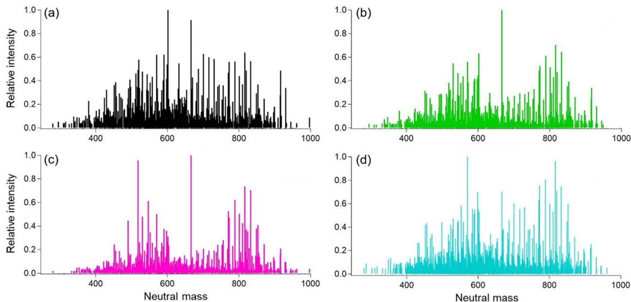
Fig. 6 Soft ionization mass spectra for the C, H, and O containing ions in the extract obtained during the smoking of different oils. The oils were heated to temperatures  $\sim 20$  °C above their smoke points. Panels (a–d) represent canola, lard, peanut, and soybean oil respectively.
